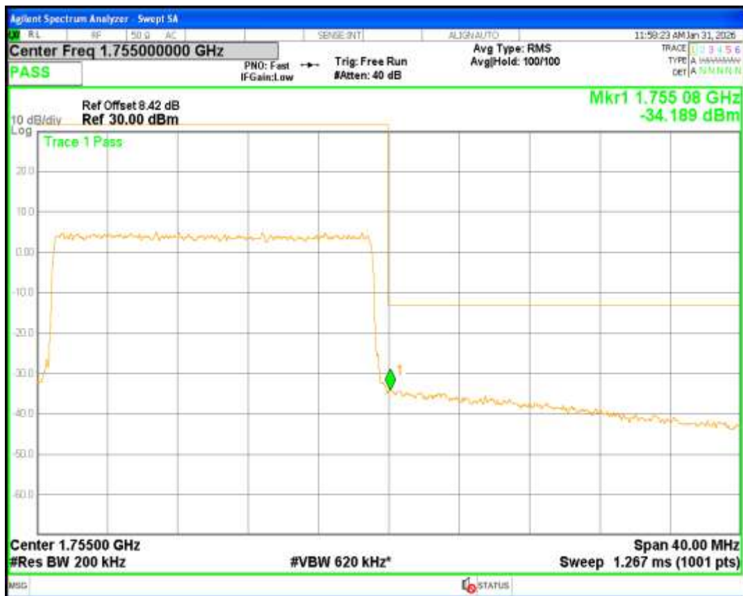
Band4 16QAM BW=3MHz Channel=19965 RB Size=15 Position=#0
