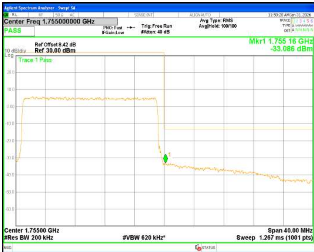
Band4 QPSK BW=3MHz Channel=19965 RB Size=15 Position=#0
