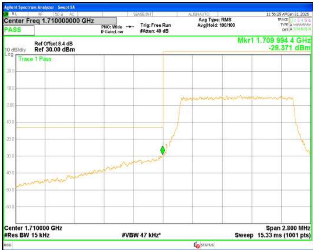
Band4 16QAM BW=1.4MHz Channel=20393 RB Size=6 Position=#0
