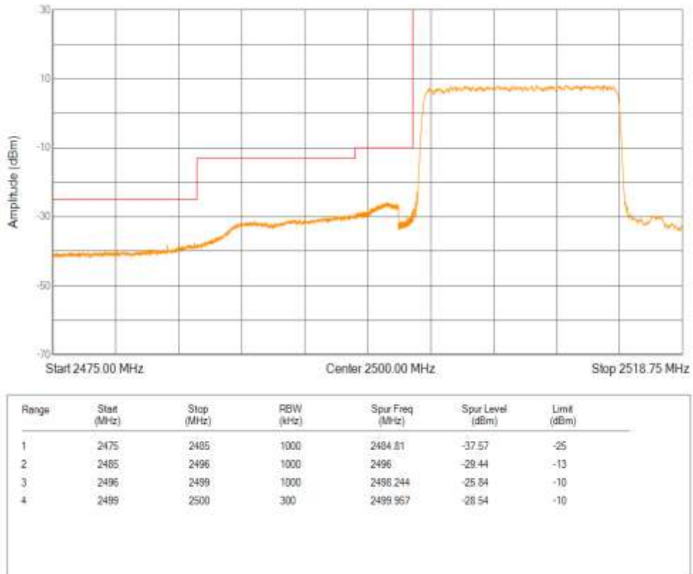
Band7 QPSK BW=15MHz Channel=21375 RB Size=75 Position=#0
