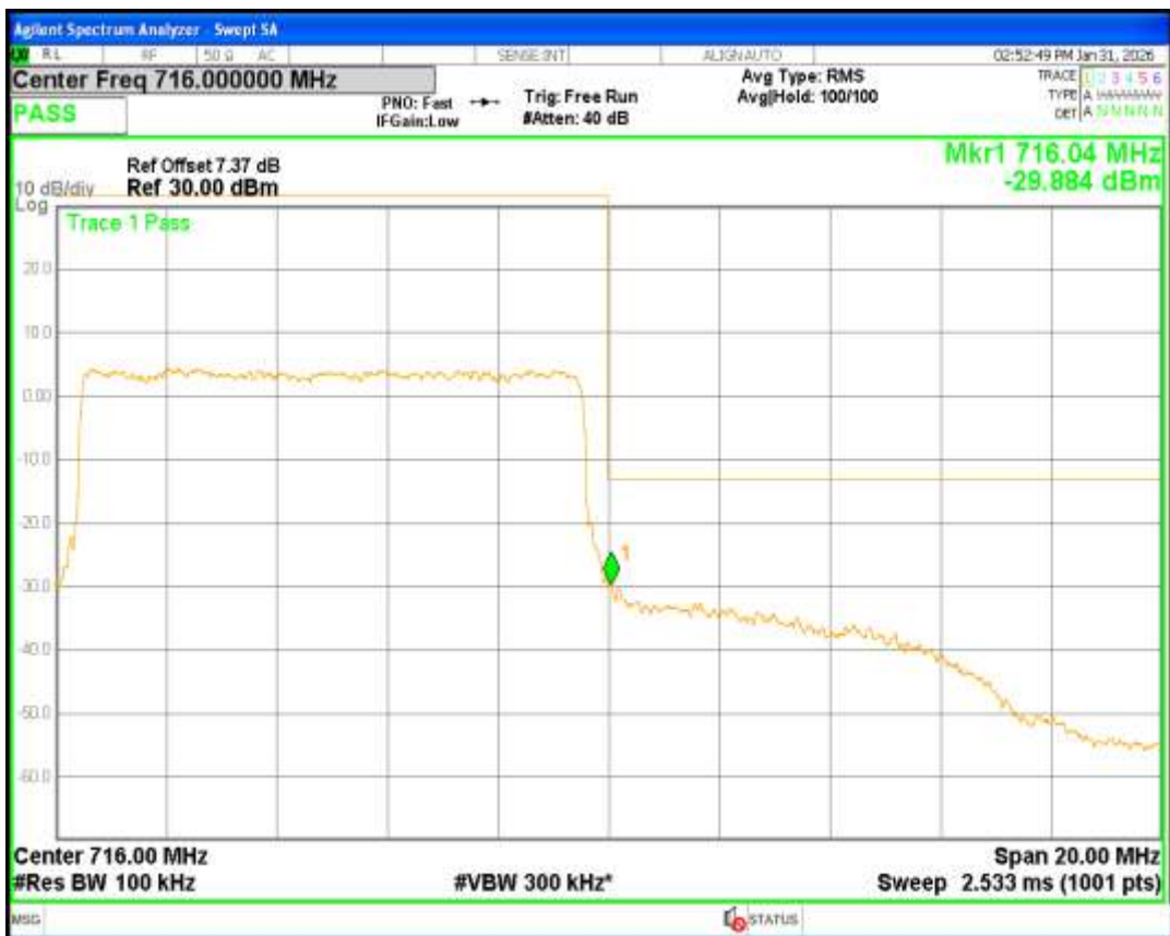
Band17 16QAM BW=5MHz Channel=23755 RB Size=25 Position=#0
