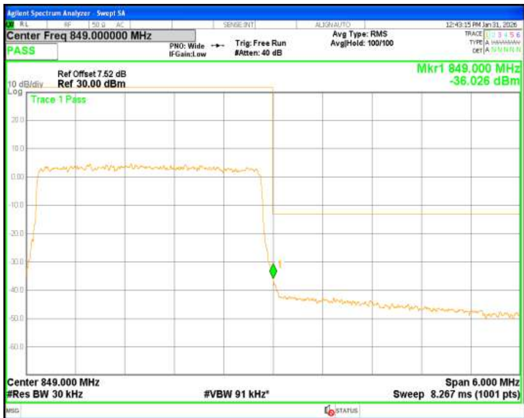
Band5 16QAM BW=5MHz Channel=20425 RB Size=25 Position=#0
