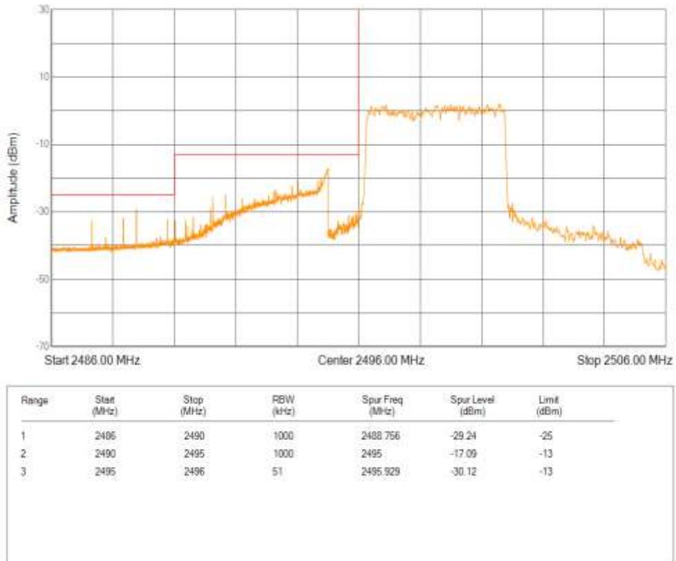
Band41 QPSK BW=5MHz Channel=41565 RB Size=25 Position=#0
