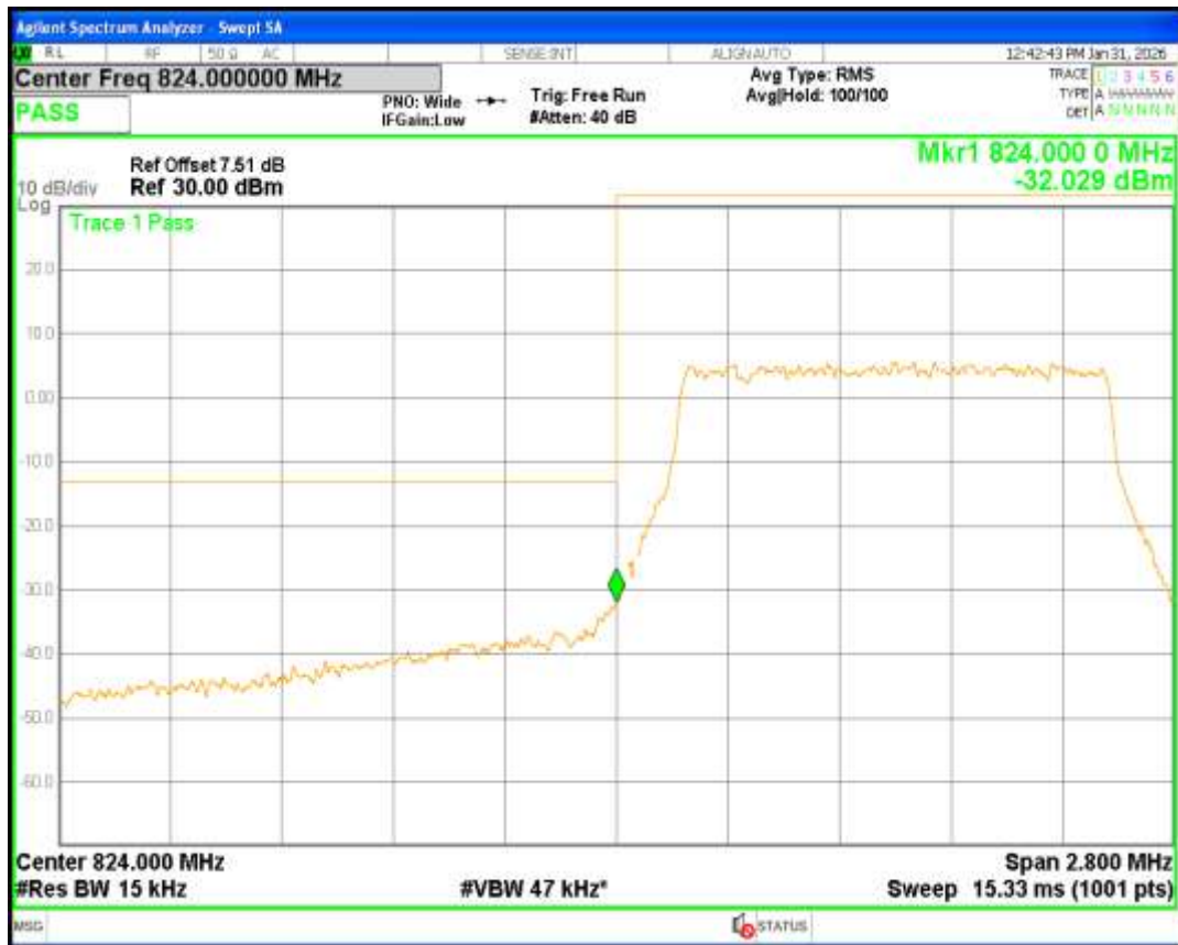
Band5 16QAM BW=1.4MHz Channel=20643 RB Size=6 Position=#0
