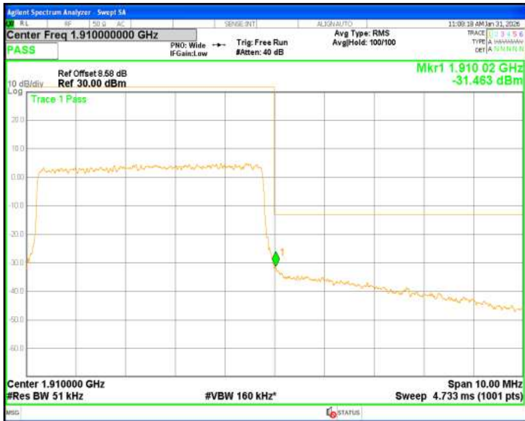
Band2 16QAM BW=5MHz Channel=18625 RB Size=25 Position=#0
