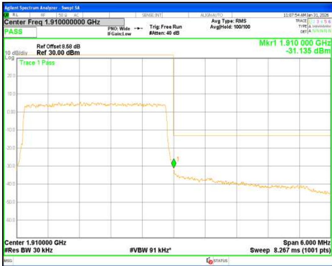
Band2 QPSK BW=5MHz Channel=19175 RB Size=25 Position=#0
