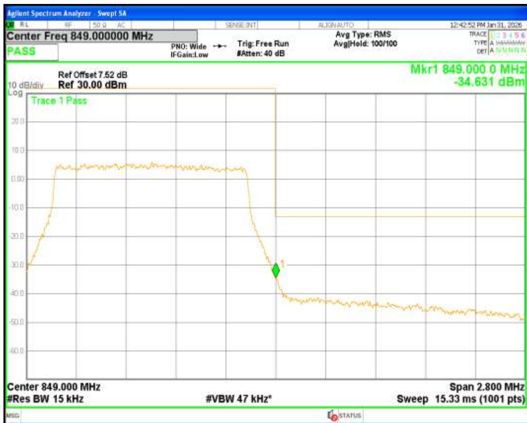
Band5 16QAM BW=10MHz Channel=20450 RB Size=50 Position=#0
