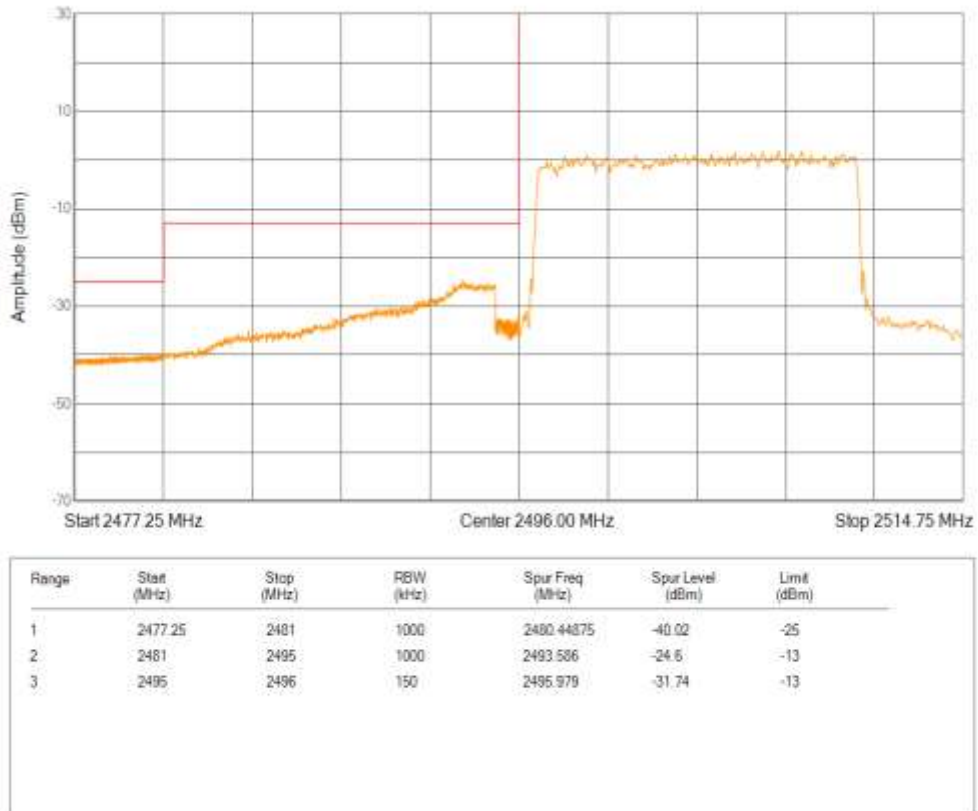
Band41 QPSK BW=15MHz Channel=41515 RB Size=75 Position=#0
