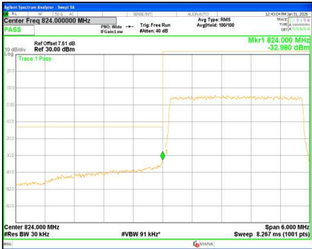
Band5 QPSK BW=3MHz Channel=20635 RB Size=15 Position=#0
