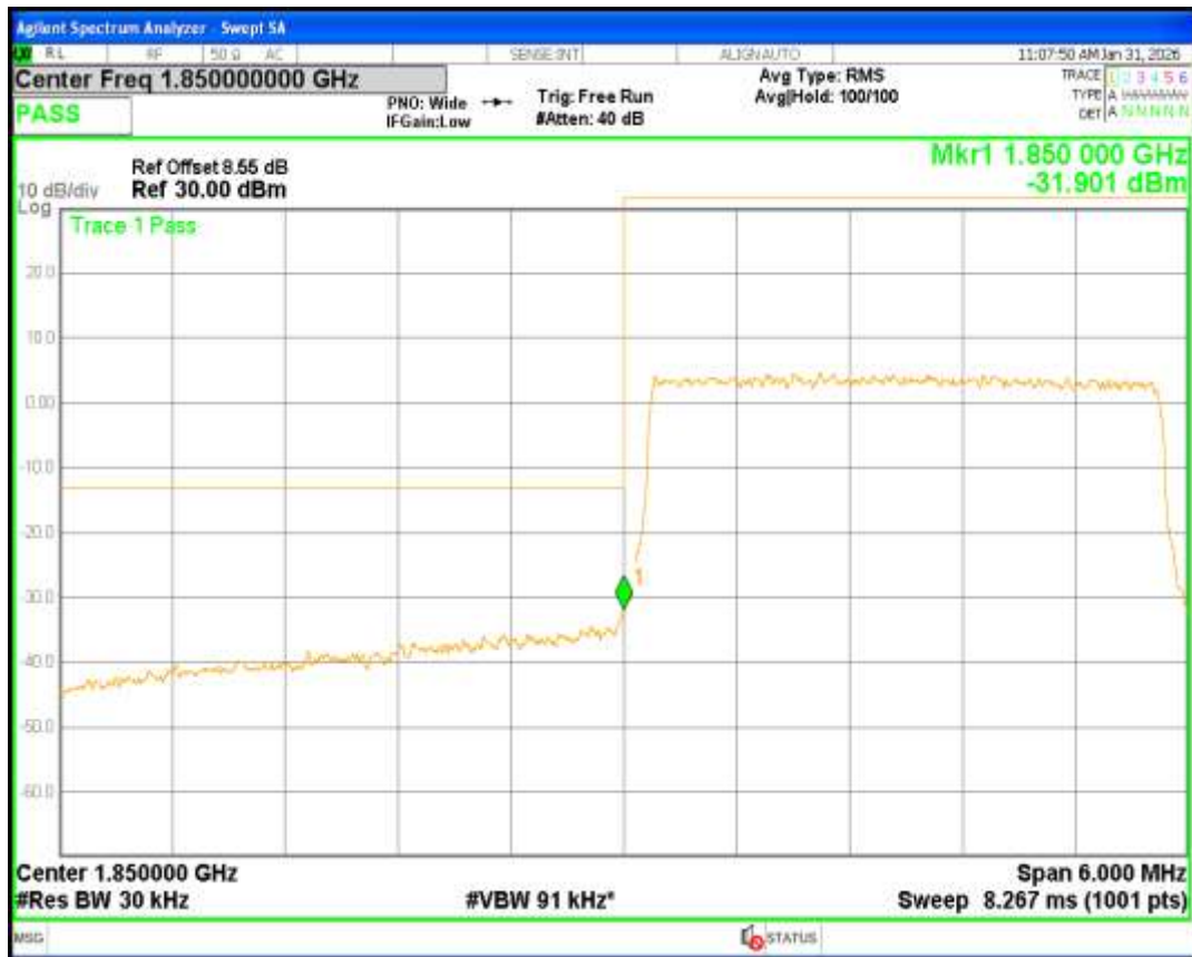
Band2 16QAM BW=3MHz Channel=19185 RB Size=15 Position=#0
