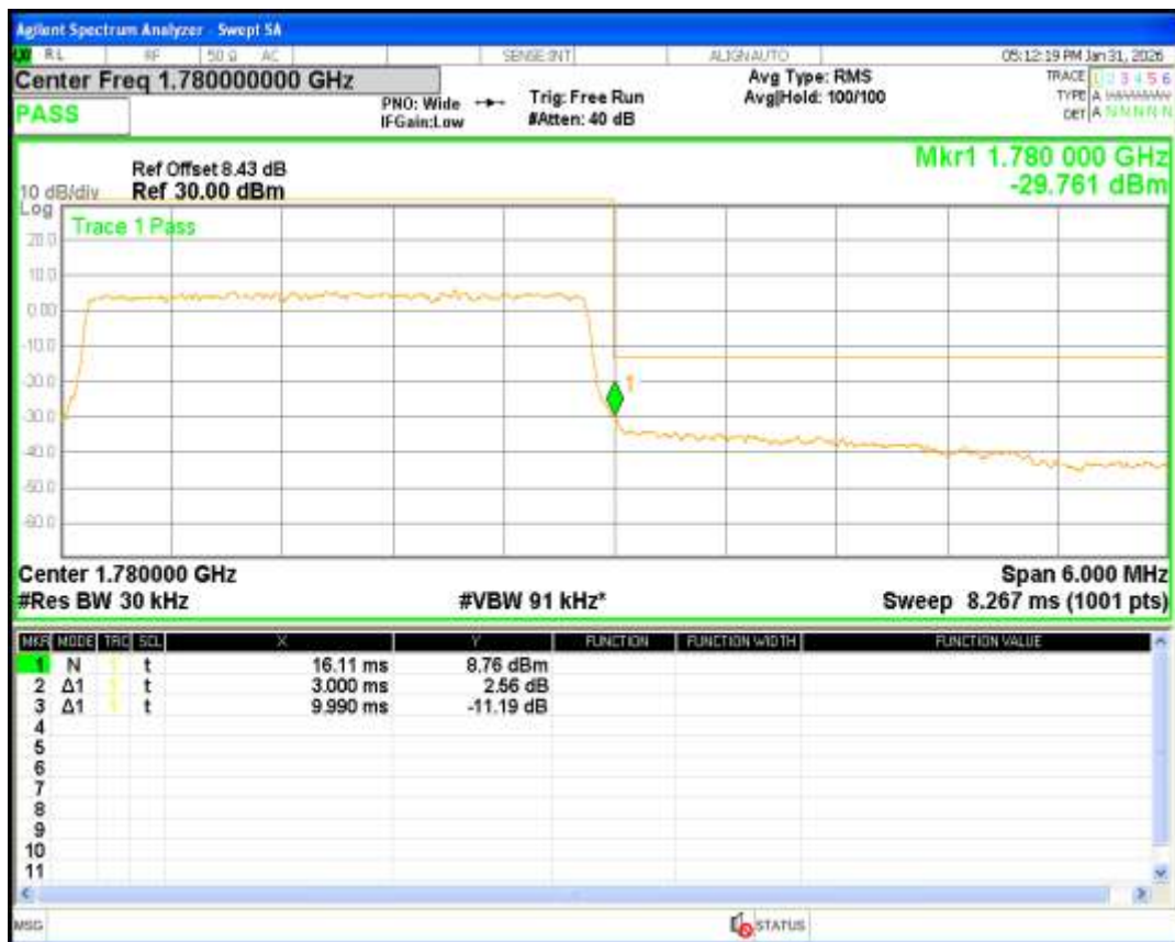
Band66 QPSK BW=5MHz Channel=131997 RB Size=25 Position=#0
