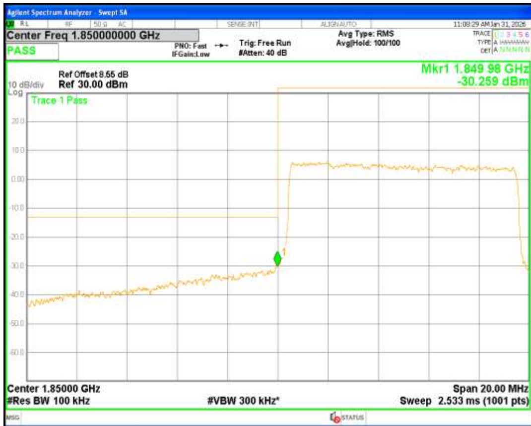
Band2 QPSK BW=10MHz Channel=19150 RB Size=50 Position=#0
