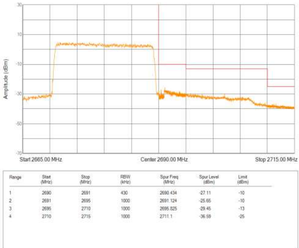
Band41 QPSK BW=5MHz Channel=39675 RB Size=25 Position=#0
