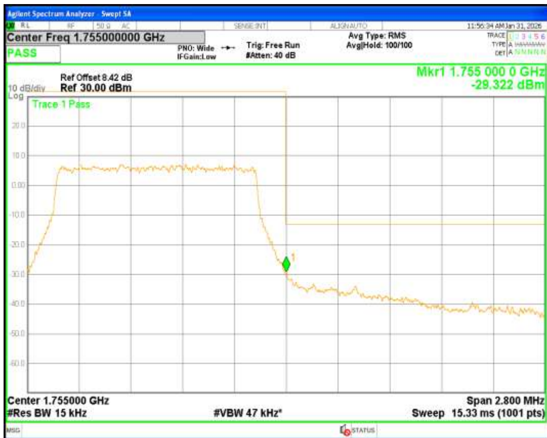
Band4 QPSK BW=10MHz Channel=20000 RB Size=50 Position=#0
