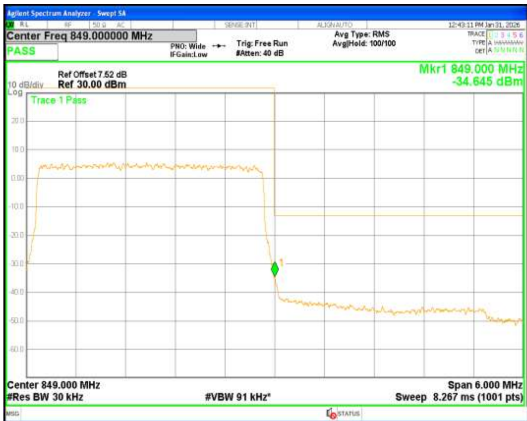
Band5 QPSK BW=5MHz Channel=20425 RB Size=25 Position=#0
