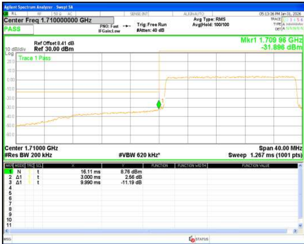
Band66 16QAM BW=20MHz Channel=132572 RB Size=100 Position=#0
