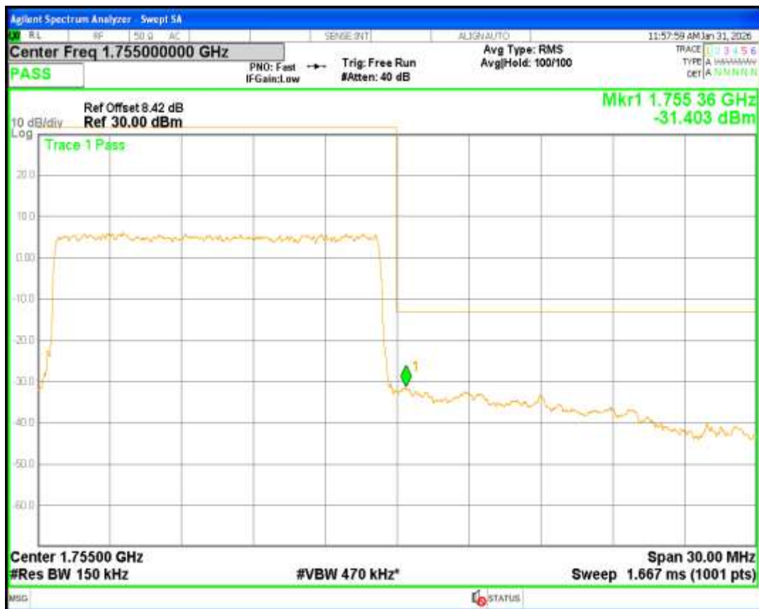
Band4 QPSK BW=20MHz Channel=20050 RB Size=100 Position=#0
