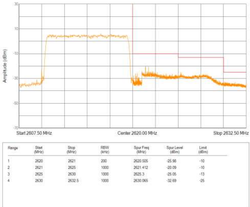
Band38 QPSK BW=15MHz Channel=37825 RB Size=75 Position=#0
