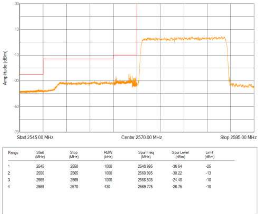
Band38 QPSK BW=20MHz Channel=38150 RB Size=100 Position=#0
