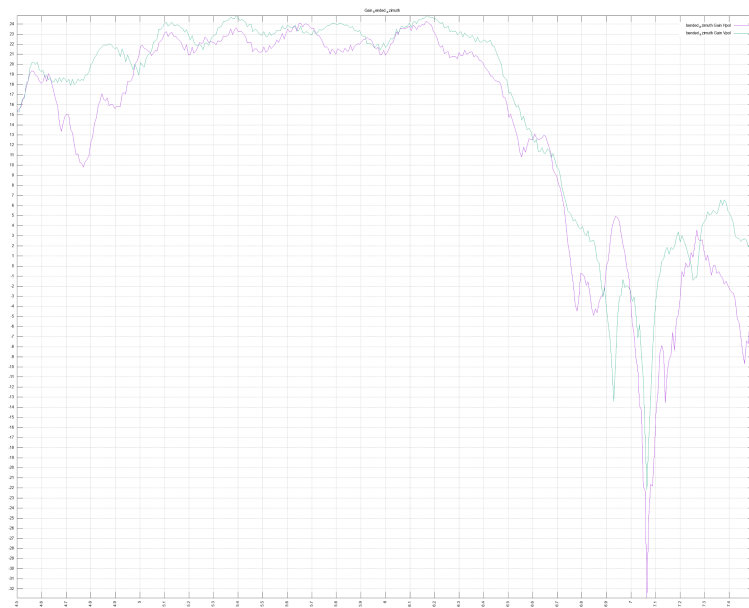
Fig.3. Measured antenna gain for H and V polarizations
