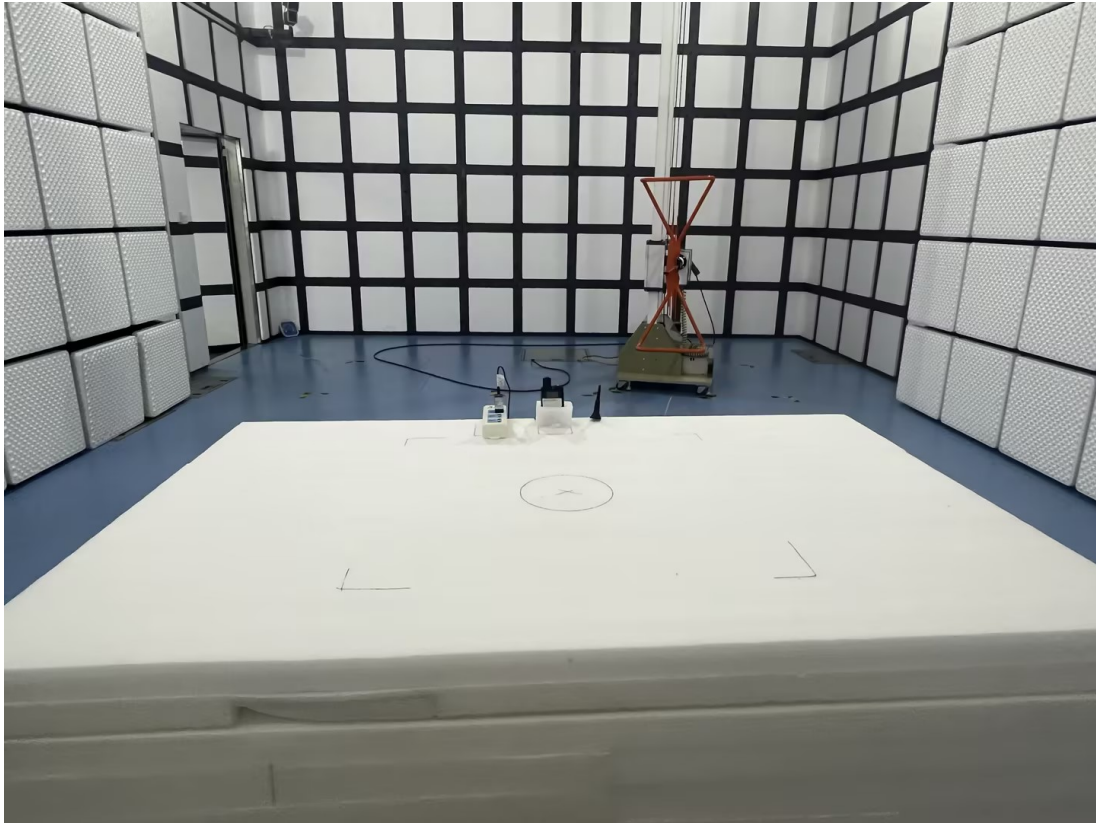
Radiation Emission - Back View (Below 1GHz)
