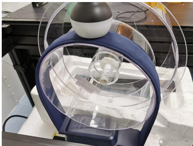
Figure 6. PN1100-S/EQ517-SS, belt fabric, Char. tube 14 mm, separation distance 0 mm
