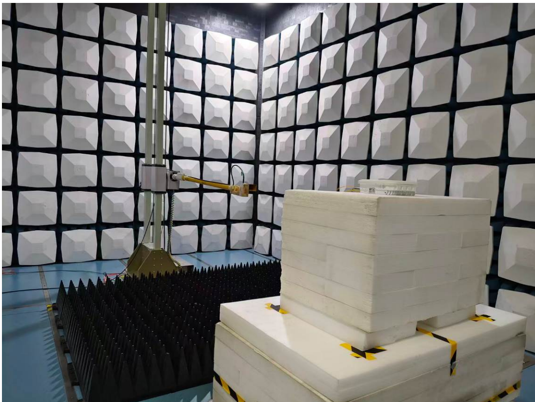
Radiated Emission 18-26.5 GHz View
