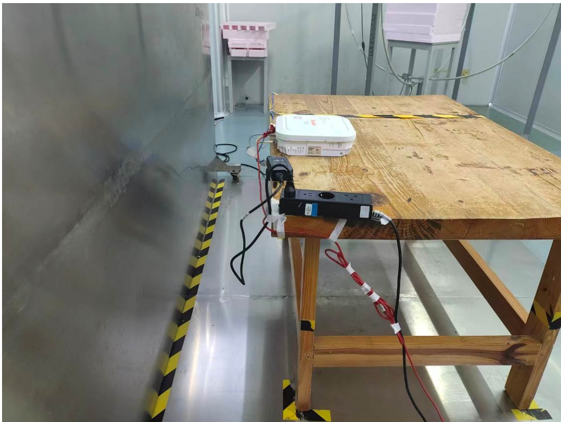
Conducted Emissions Side View
