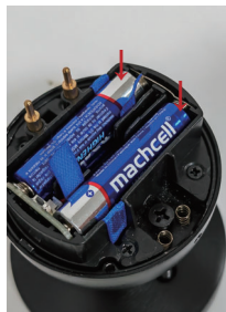
11. Install two more batteries
