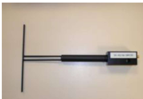
Figure 1 – MVG COMOSAR Validation Dipole
