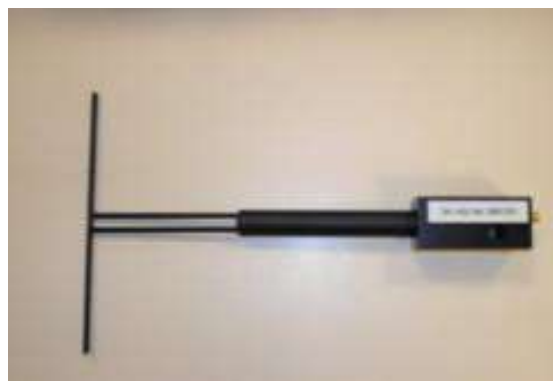
Figure 1 – MVG COMOSAR Validation Dipole
