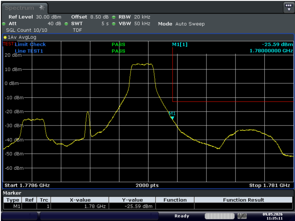
Test_Graph_band66_1779.3MHz_1.4M_16QAM_1RB#HIGH_Band edge
