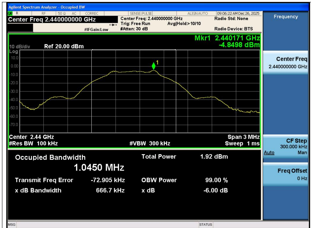
Test_Graph_LE1M_ANT1_2440_1Mbps_DTSBW
