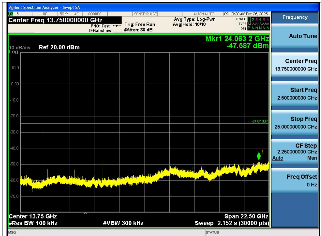
Test_Graph_LE1M_ANT1_2480_1Mbps_Higher Band Emissions
