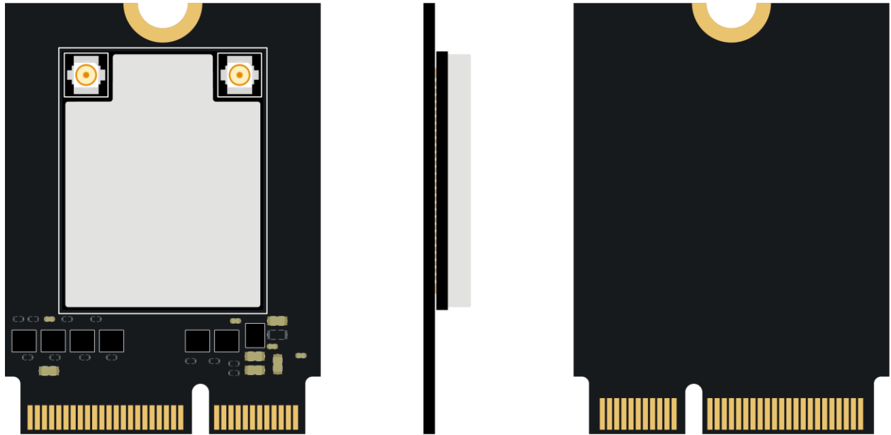
Figure 1 M.2 KEY E 2230 Module View
