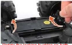
Rotate the locking buckles on both sides to remove the battery cover
