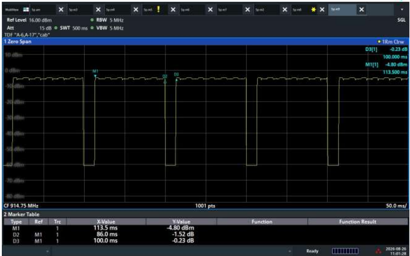
Figure 7-1 900 MHz Band RFID Transmission Plot
