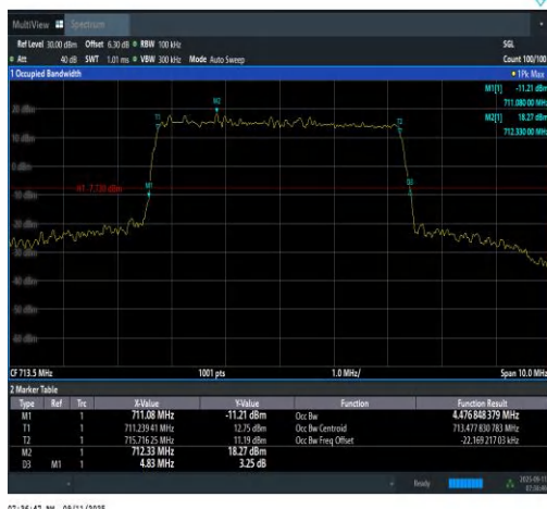
Band12-5MHz-QPSK-23155-25RB#0-PASS
