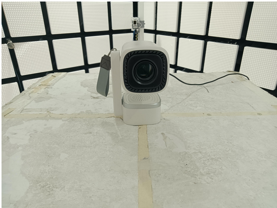
Radiated spurious emission Test Setup-3(Above 18GHz)
