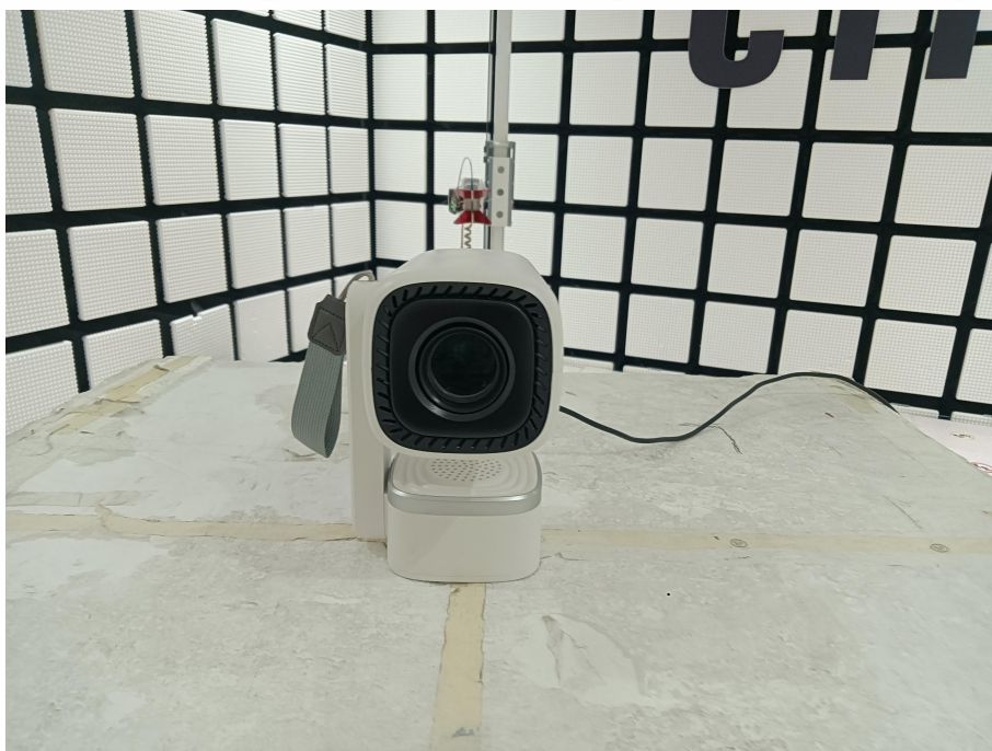
Radiated spurious emission Test Setup-2(Above 1GHz)
