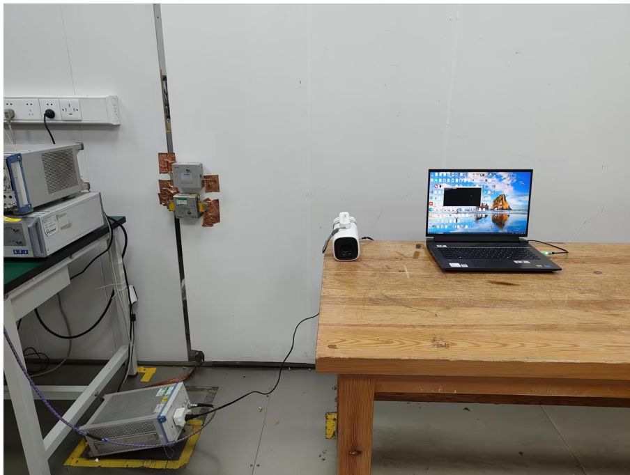
Conducted Emissions Test Setup
