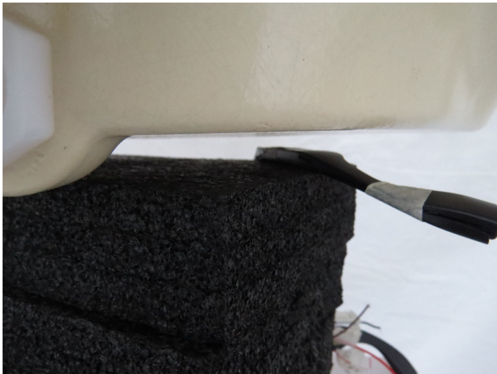
Picture 1: Back Side, the distance from EUT to the bottom of the Phantom is 6mm
