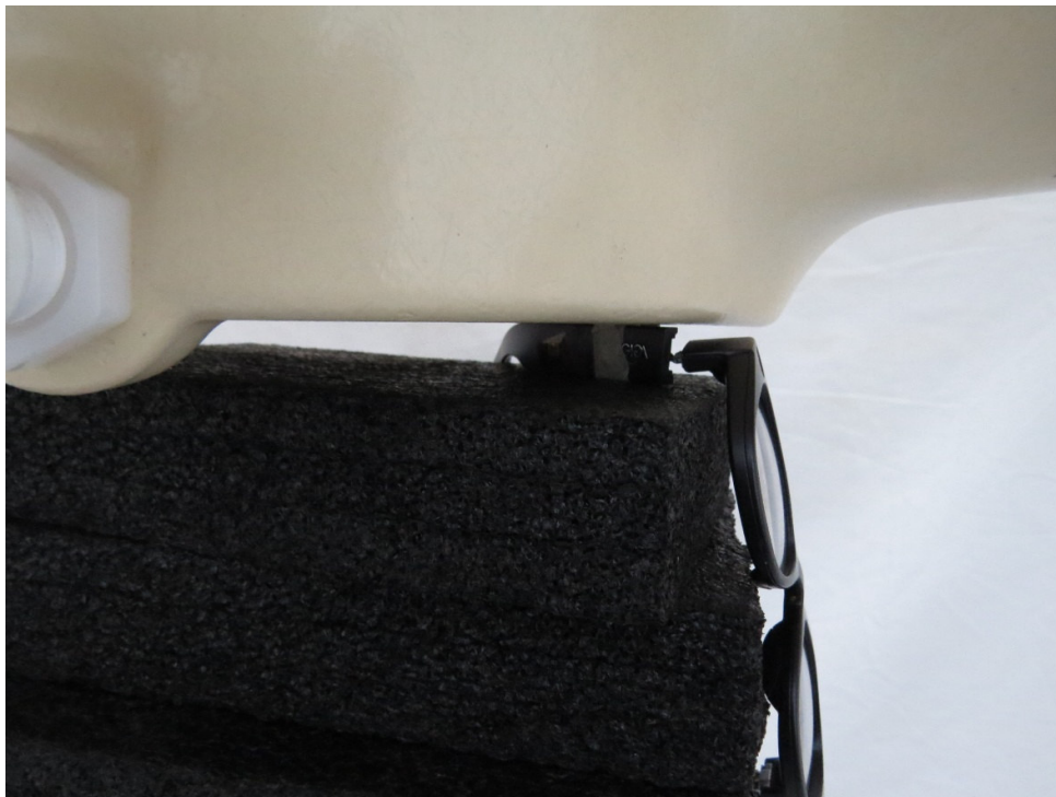
Picture 3: Left Edge, the distance from EUT to the bottom of the Phantom is 0mm
