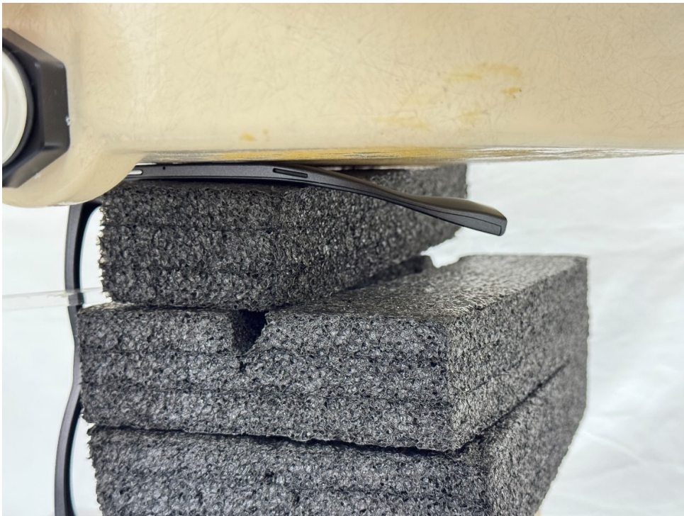
Picture 6: Back Side, the distance from EUT to the bottom of the Phantom is 0mm
