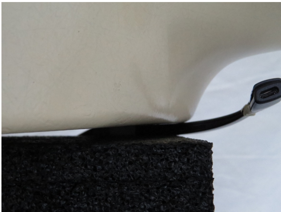
Picture 2: Front Side, the distance from EUT to the bottom of the Phantom is 0mm
