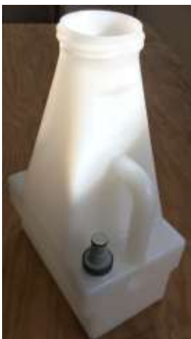
Figure 12-1: Intermediate tank with quick connector
