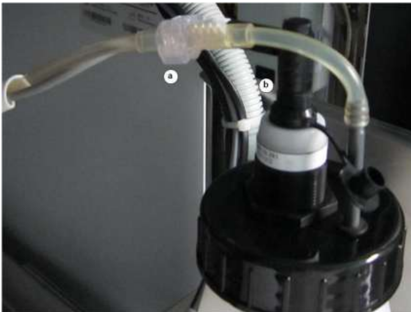
Figure 12-7: Wash buffer intermediate tank connectors
