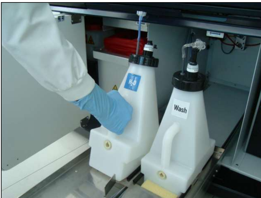
Figure 8-12: Intermediate tank raised up and removed
