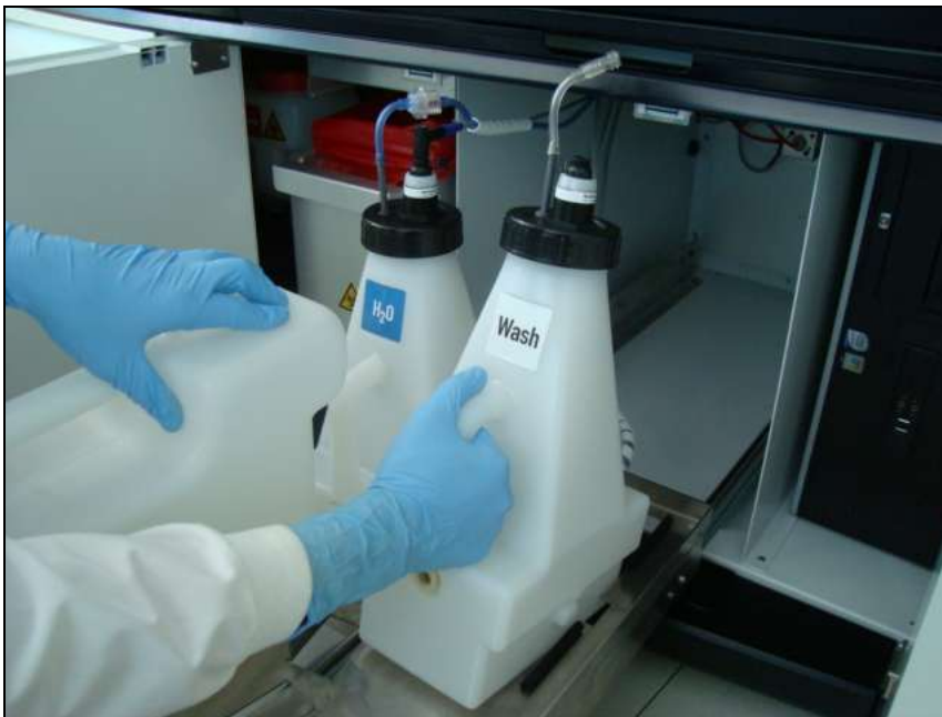
Figure 8-8: Wash buffer intermediate tank raised up and removed
