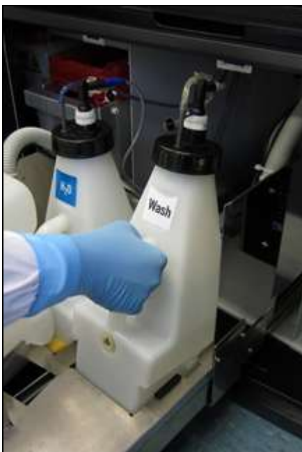
Figure 12-9: Wash buffer intermediate tank raised up and removed
