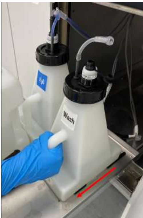
Figure 8-7: Wash buffer intermediate tank moved to the front
