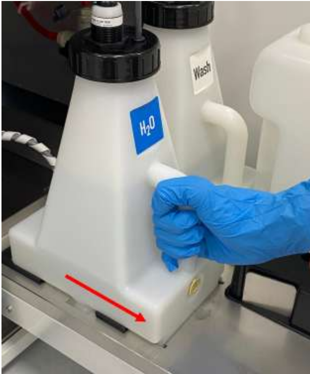
Figure 8-11: Intermediate tank moved to the front
