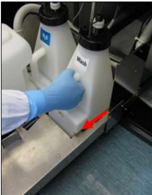
Figure 12-8: Wash buffer intermediate tank moved to the front
