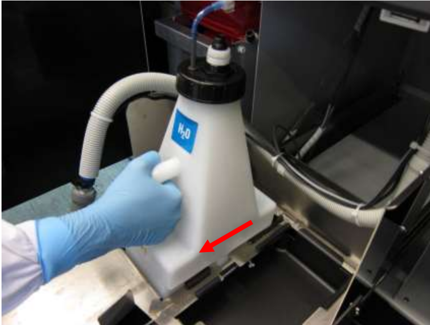
Figure 12-13: Intermediate tank moved to the front
