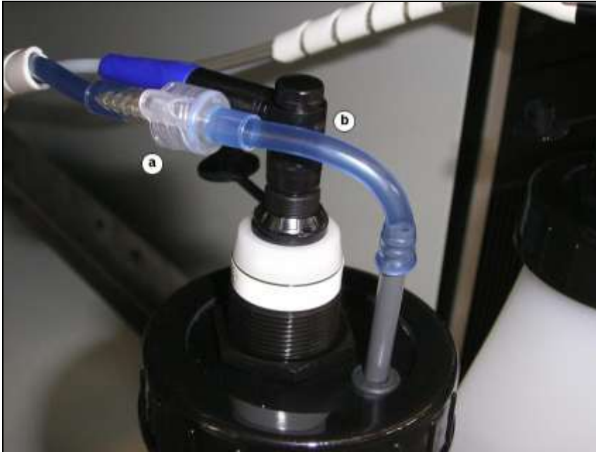
Figure 8-10: Water intermediate tank connectors
