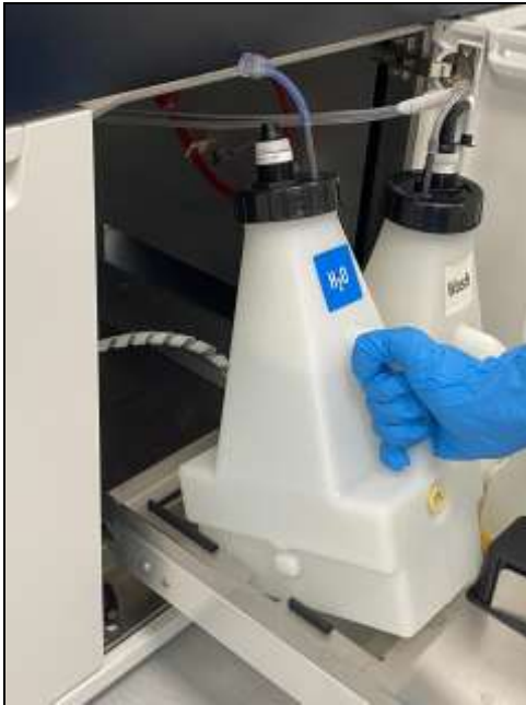
Figure 8-12: Intermediate tank raised up and removed
