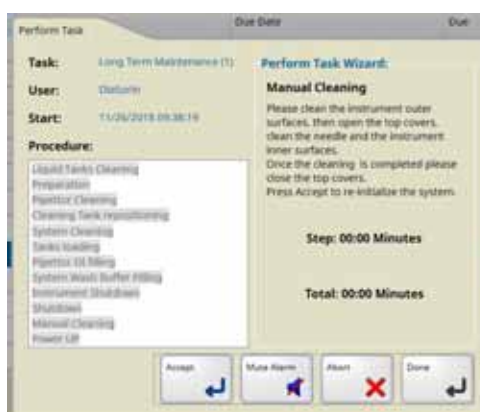
Figure 7–3: Long Term Maintenance - Manual Cleaning pop-up
