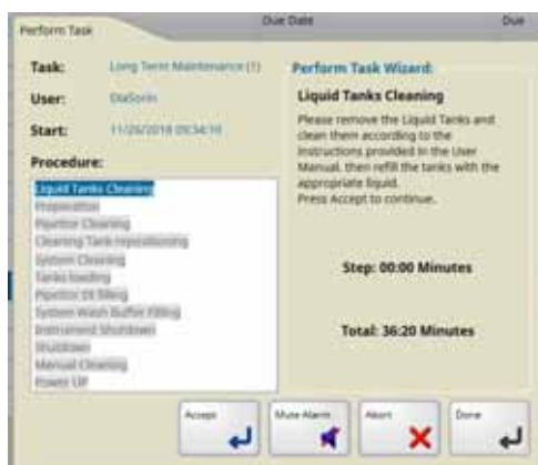
Figure 7–1: pop-up of the instruments tanks cleaning
