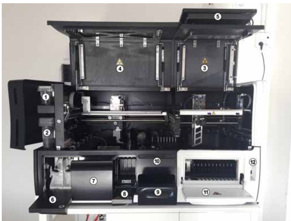
Figure 4-2: LIAISON ® XS flaps and drawers
