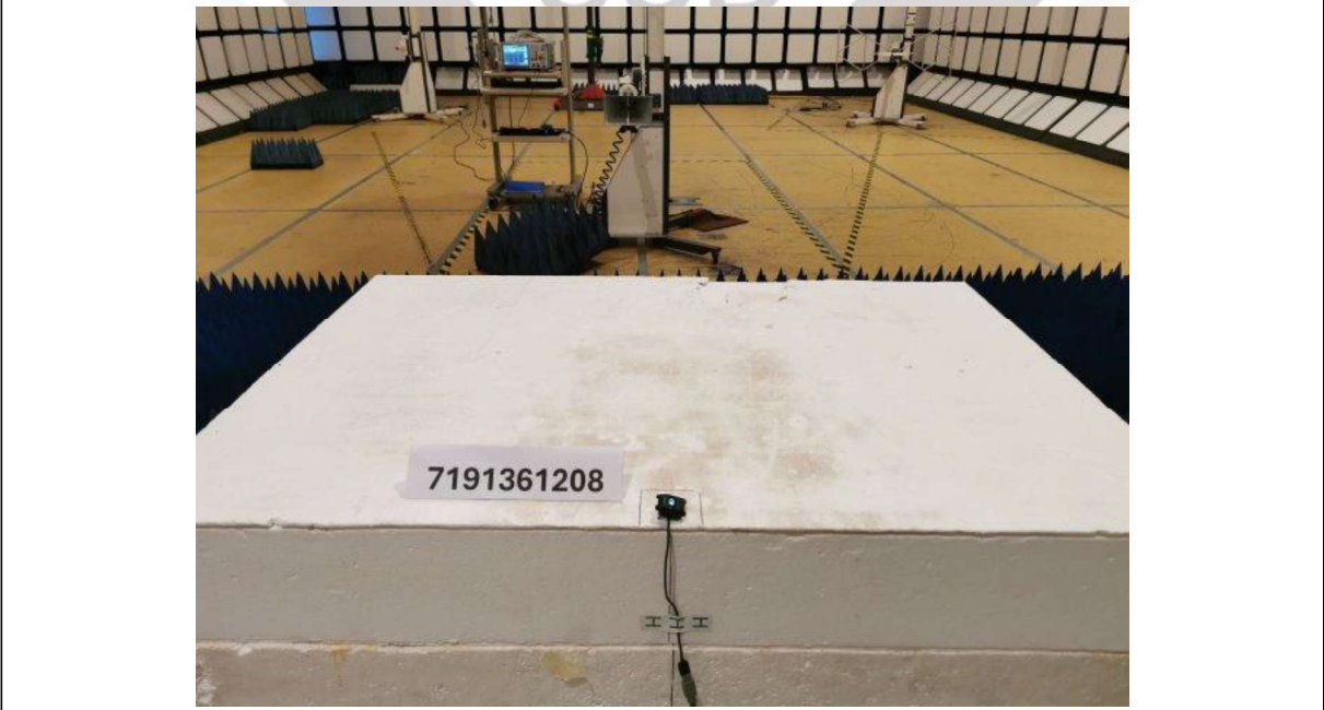
Radiated Emissions (Spurious Emissions Inclusive Restricted Bands Requirement) Test Setup (Rear View)
