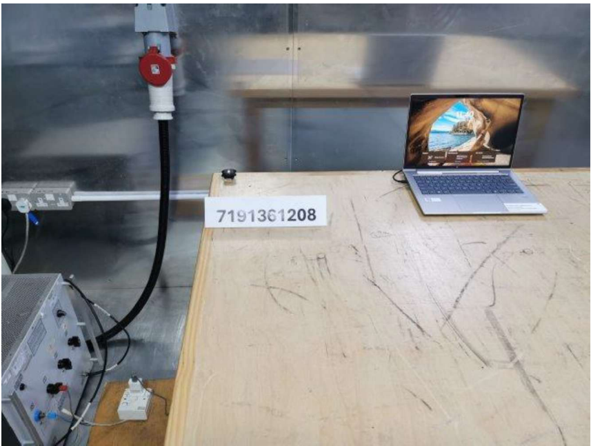
Conducted Emissions Test Setup (Front View)
