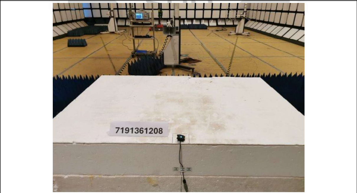
Band Edge Compliance (Radiated) Test Setup
