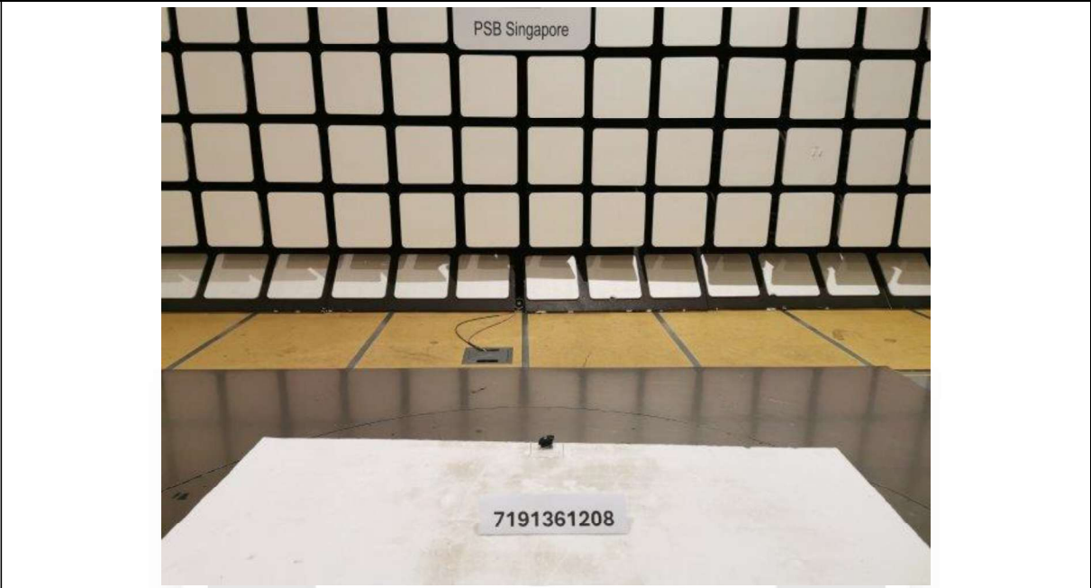
Radiated Emissions (Spurious Emissions Inclusive Restricted Bands Requirement) Test Setup (Front View)
