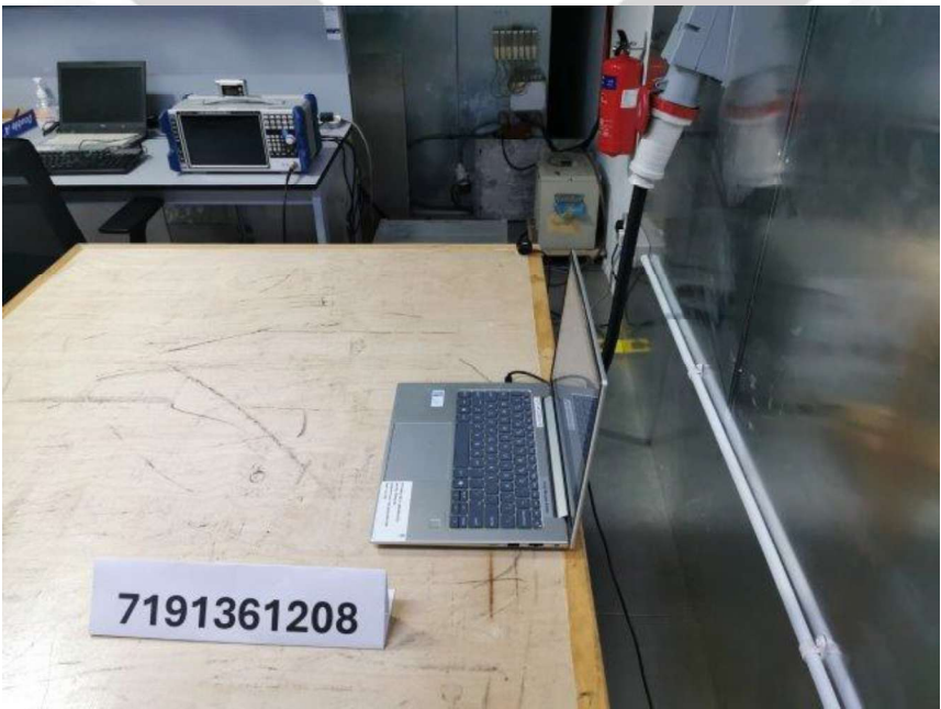
Conducted Emissions Test Setup (Rear View)
