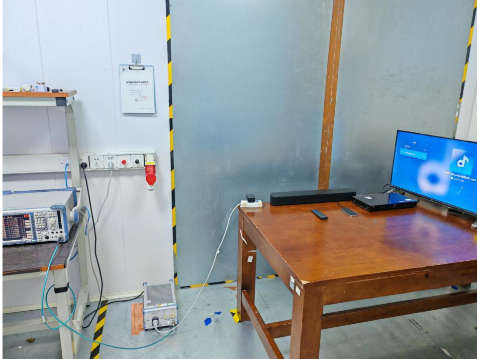
Conducted emissions at AC power line (150kHz-30MHz)
