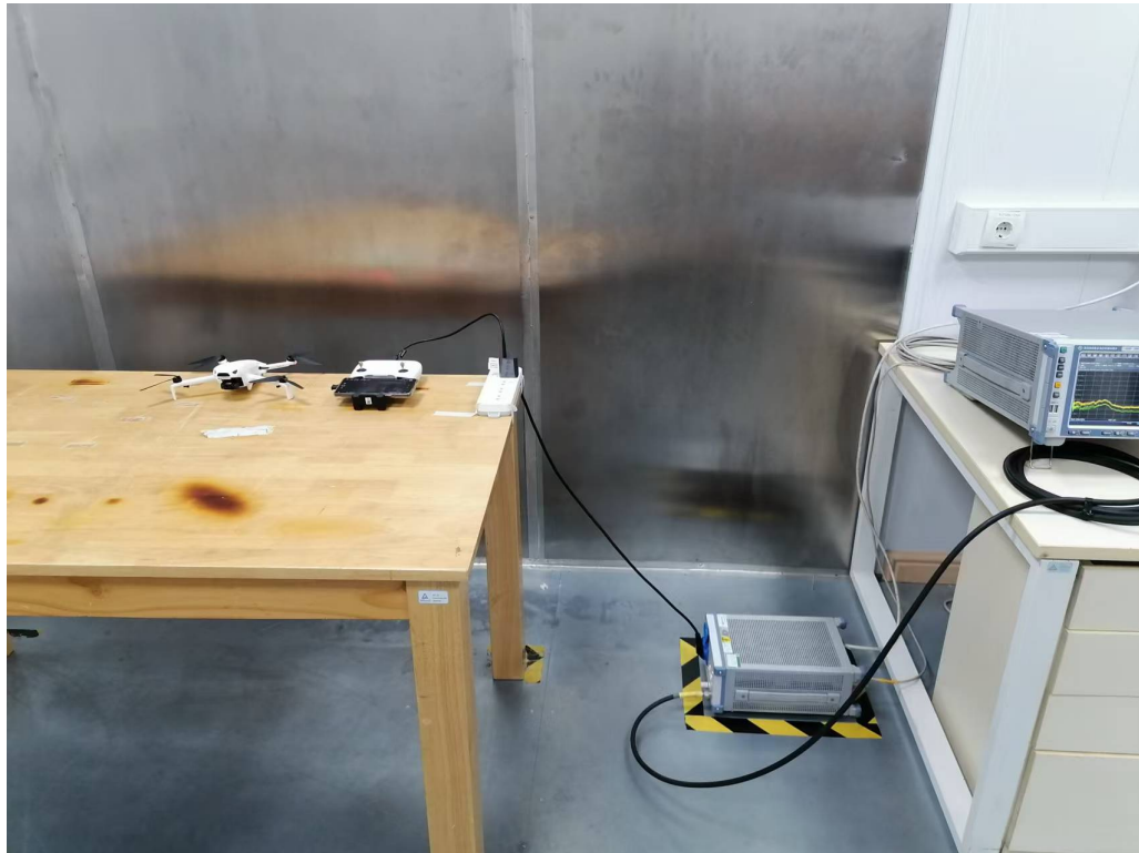
Photograph 3: Set-up for Conducted Emission on AC Mains
