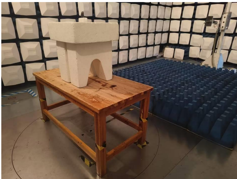
Test Setup For Radiated Emission (Above 1GHz)
