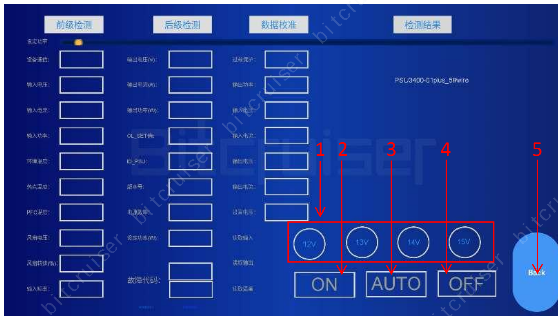
Fig 5.44 — Illustration of Avalon Power Supply Test Interface Function Button
