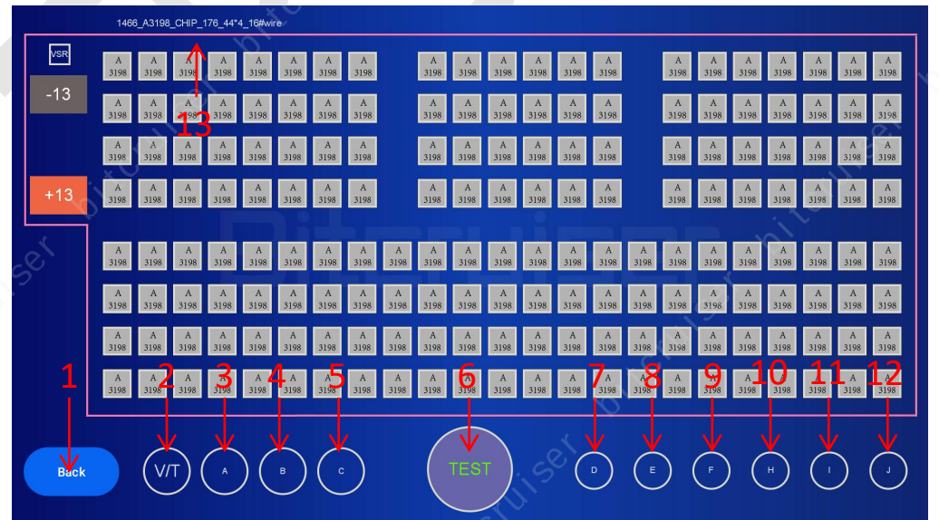
Fig 5.37 — Illustration of Avalon Hashboard Test Function Buttons
