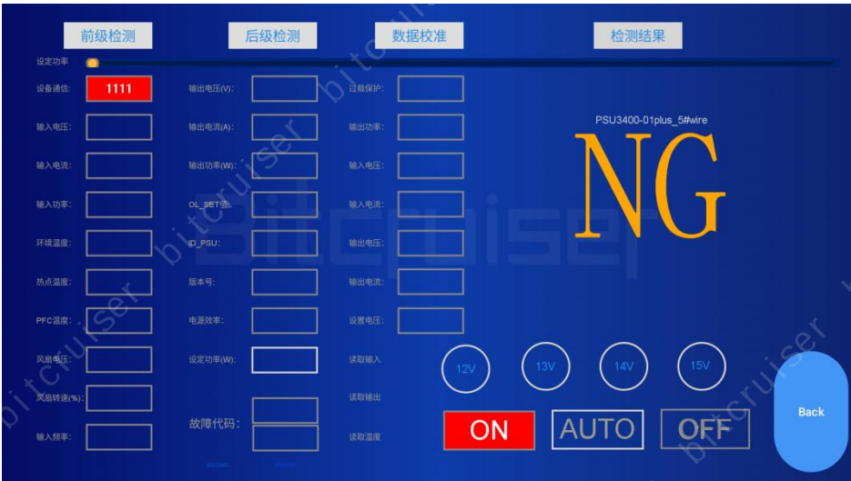
Fig 5.45 — Illustration of a Failed Avalon Power Supply Test (Part 1)
