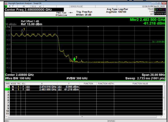
Out Of Band Emission(Right) \pi/4 DQPSK_2-DH5_Channel Hopping
