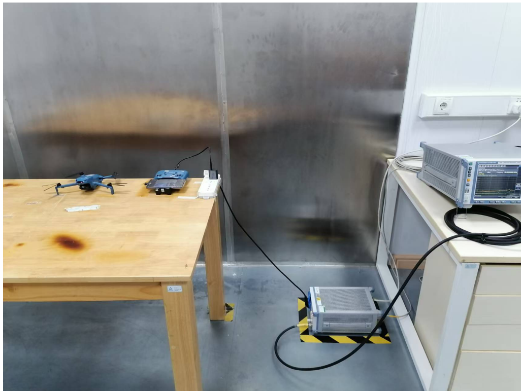
Photograph 3: Set-up for Conducted Emission on AC Mains
