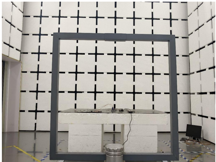
Radiation Emission Test Setup (Below 30MHz)
