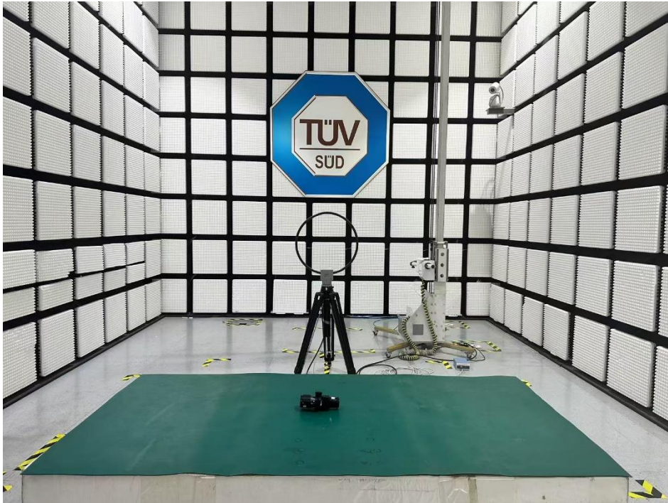
Radiated Emission Setup 9kHz ~ 30MHz
