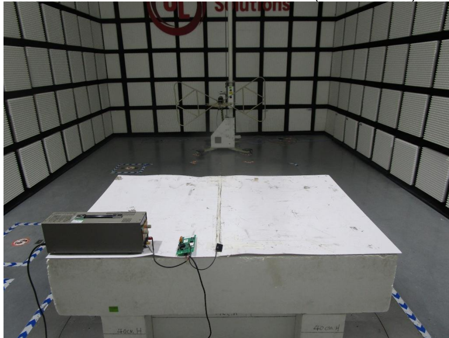
RADIATED RF MEASUREMENT SETUP (30MHz~1GHz)
