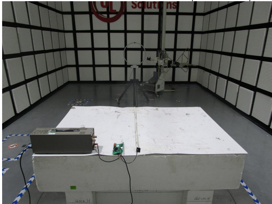
RADIATED RF MEASUREMENT SETUP (Below 30MHz)
