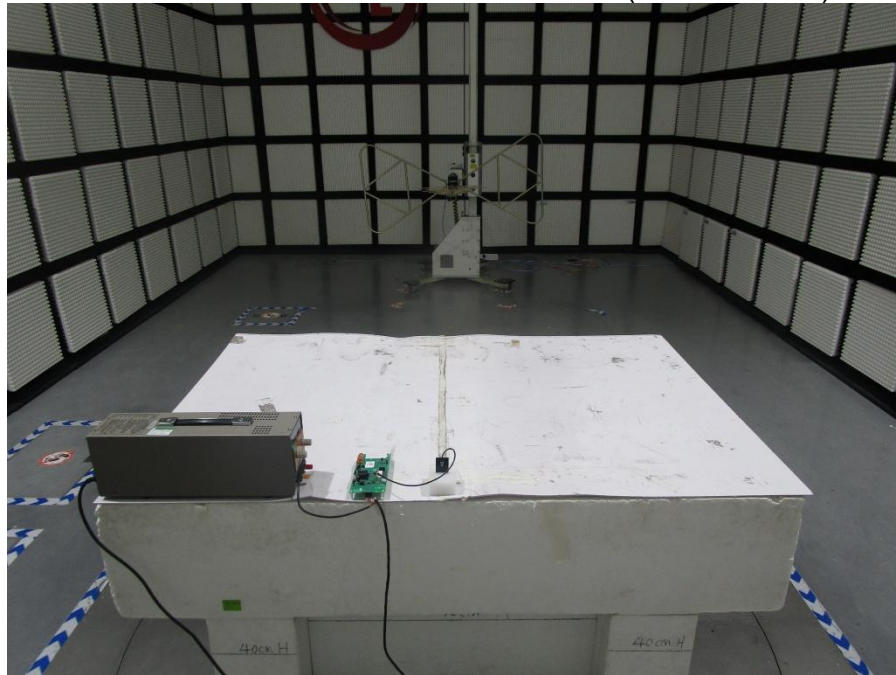
RADIATED RF MEASUREMENT SETUP (30MHz~1GHz)
