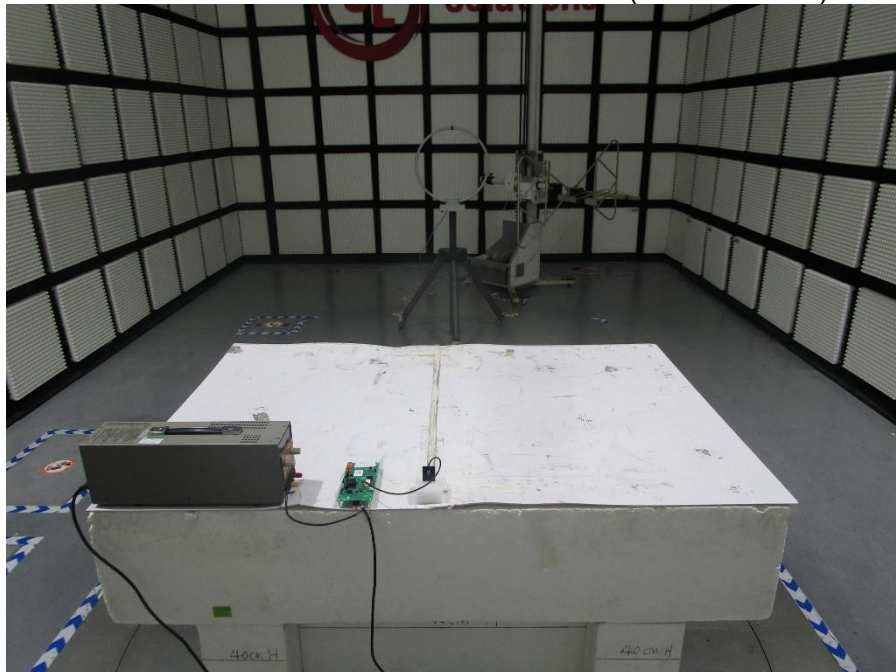
RADIATED RF MEASUREMENT SETUP (Below 30MHz)
