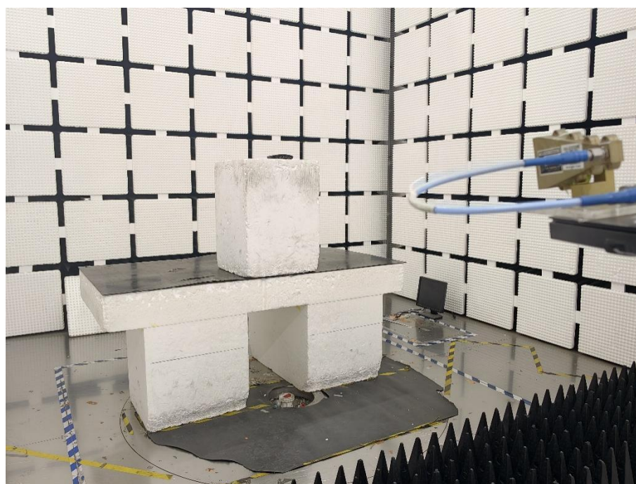
Radiation Emission Test Setup (Above 18GHz)
