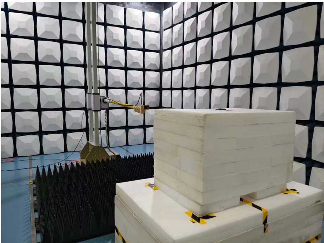
Radiated Emission 18-25 GHz View
