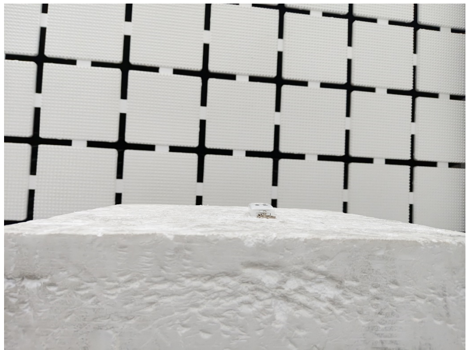
Radiation Emission Test Setup (close up)
