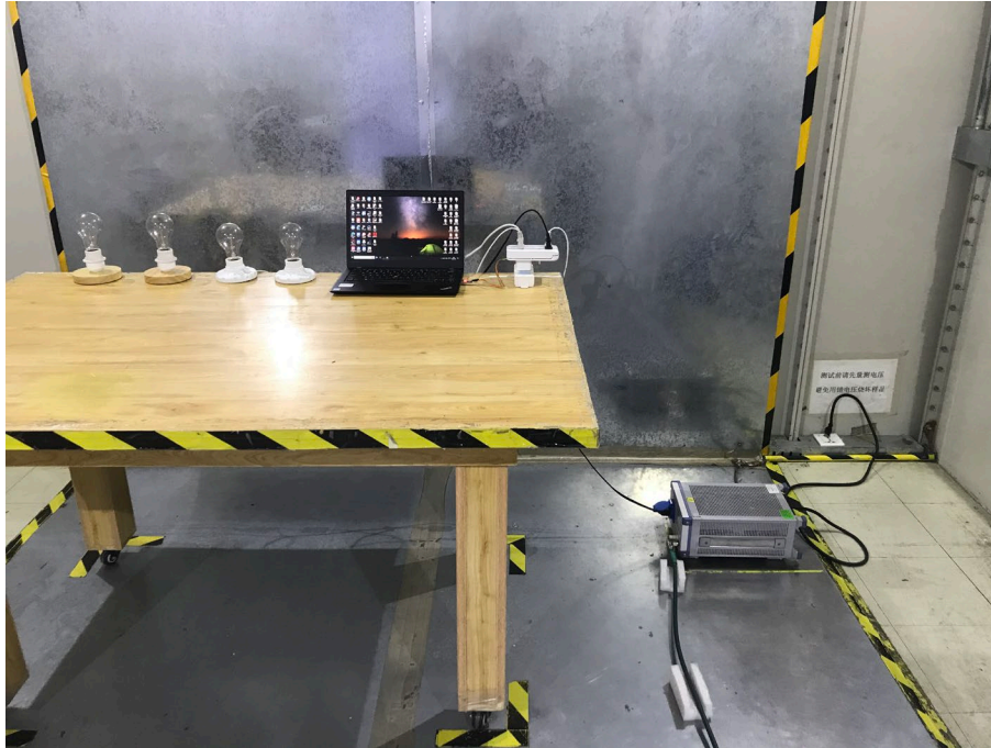
Conducted Emissions - Left View
