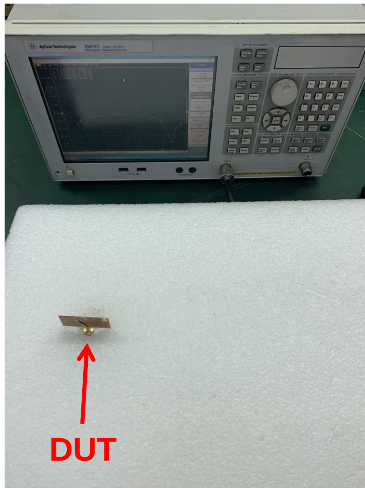
FIGURE4.1.1 ANTENNA LOADED WITH REFERENCE PCB TESTED WITH VNA E5071C
