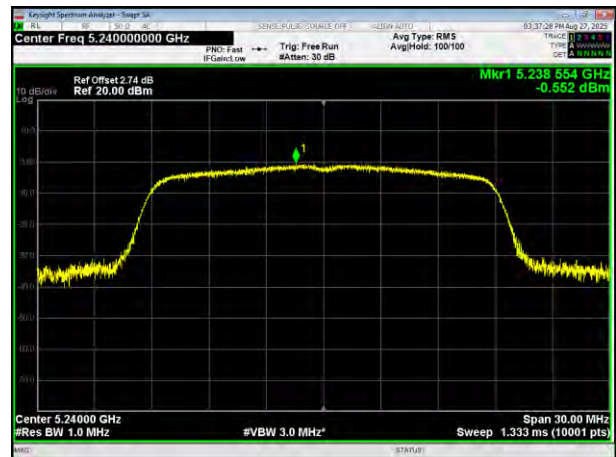
(802.11n20) PSD plot on channel 48
