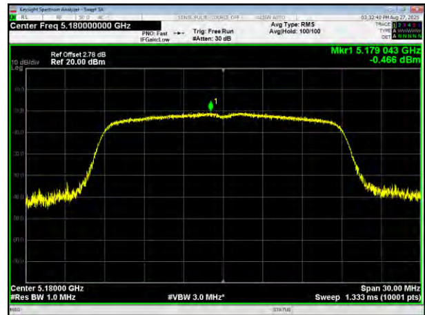
(802.11n20) PSD plot on channel 48
