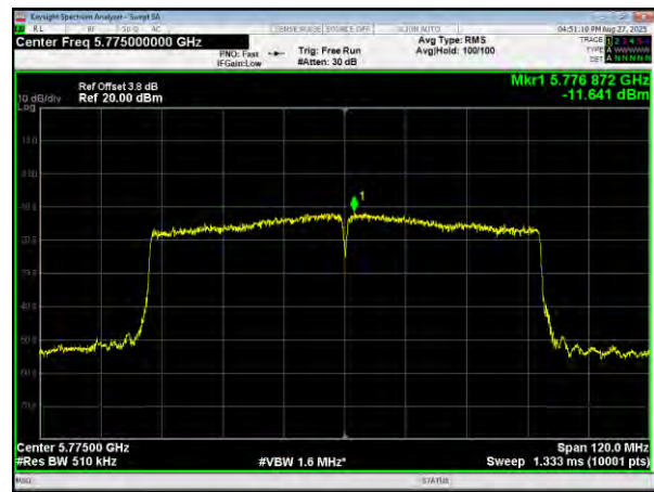
(802.11ac80) PSD plot on channel 155
