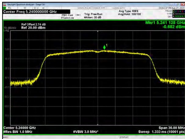
(802.11ac20) PSD plot on channel 48
