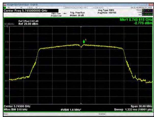
(802.11n20) PSD plot on channel 149
