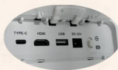
Type-C/HDMI/USB/DC-12V/Power supply mode switch button
