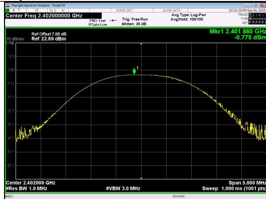
Peak Output Power BLE 1M_Channel 0
