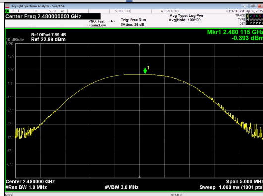
Peak Output Power BLE 1M_Channel 39
