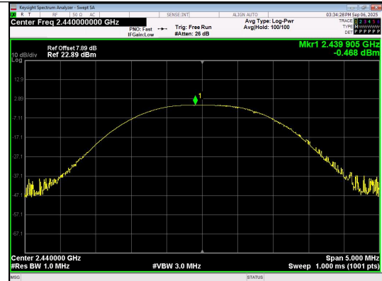
Peak Output Power BLE 1M_Channel 19
