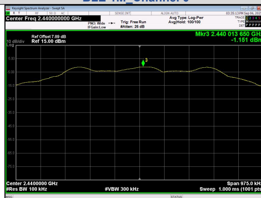
In-Band Reference Level BLE 1M_Channel 19
