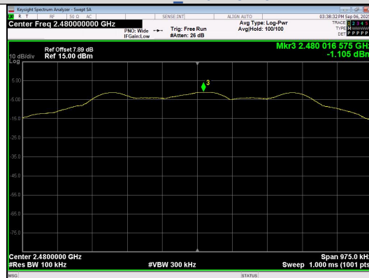
In-Band Reference Level BLE 1M_Channel 39
