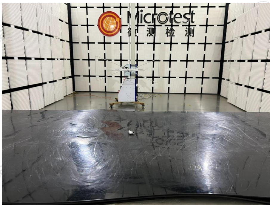
Radiated emissions (below 1GHz)
