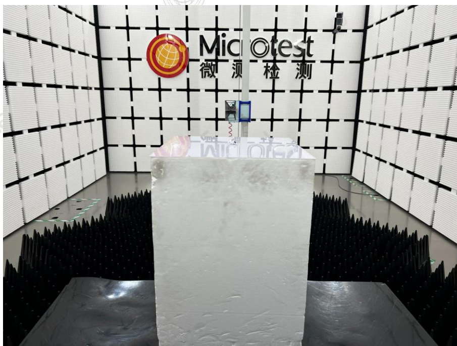
Radiated emissions (above 1GHz)
