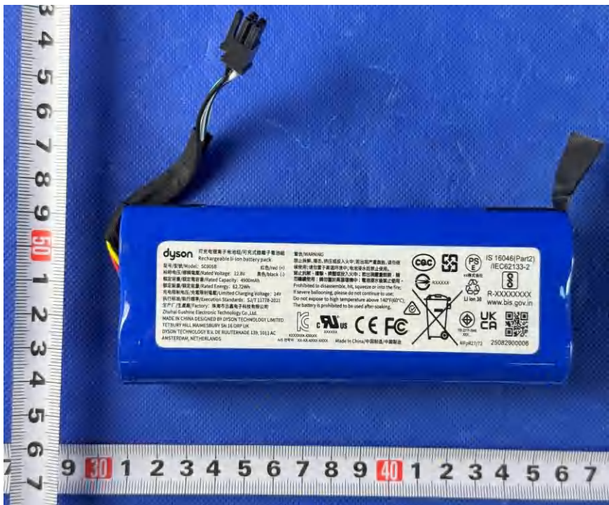
Figure 12. Li-ion battery pack
