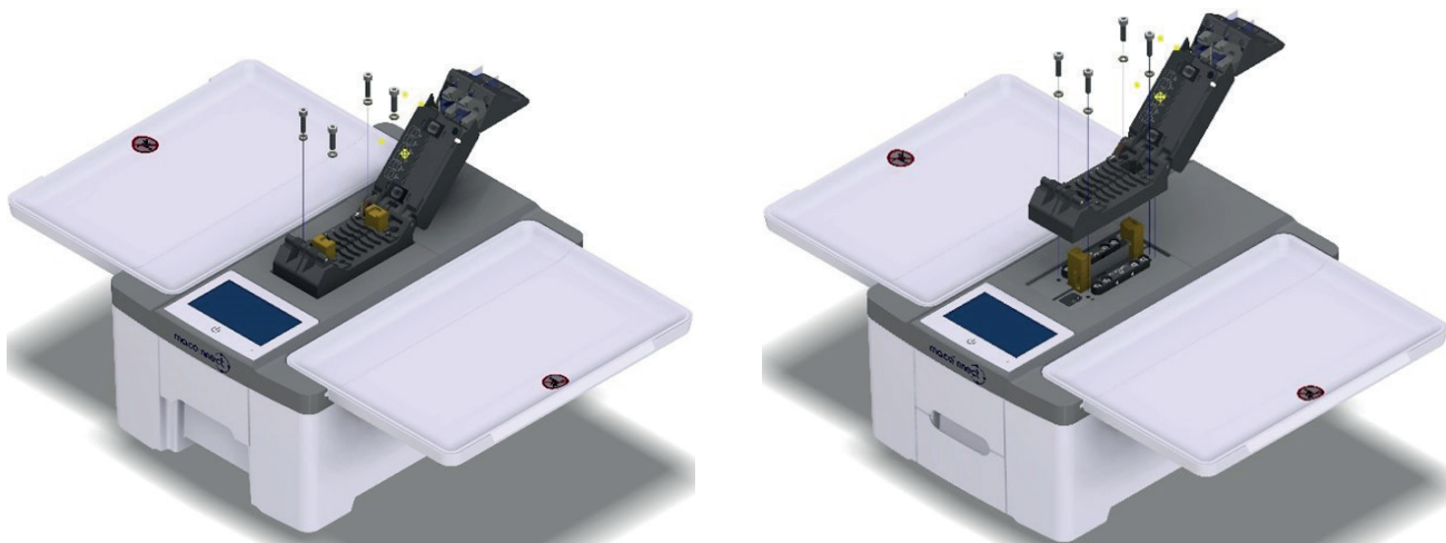
Figure 47. Dismantling of the tube holder
