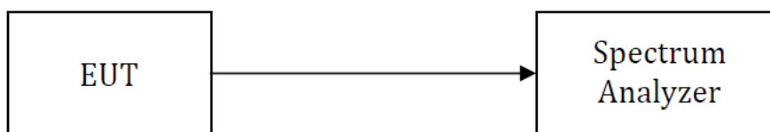
Test Setup Block Diagram
