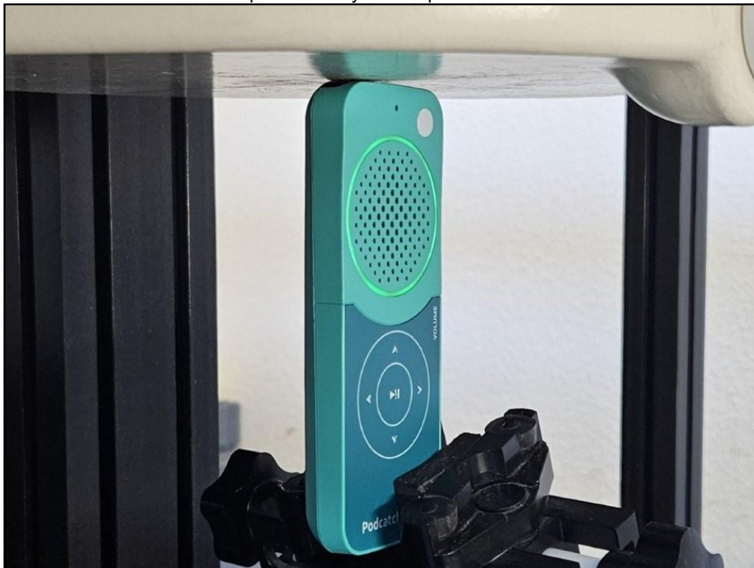
Photo 19: Test position body worn top side with 0 mm distance
