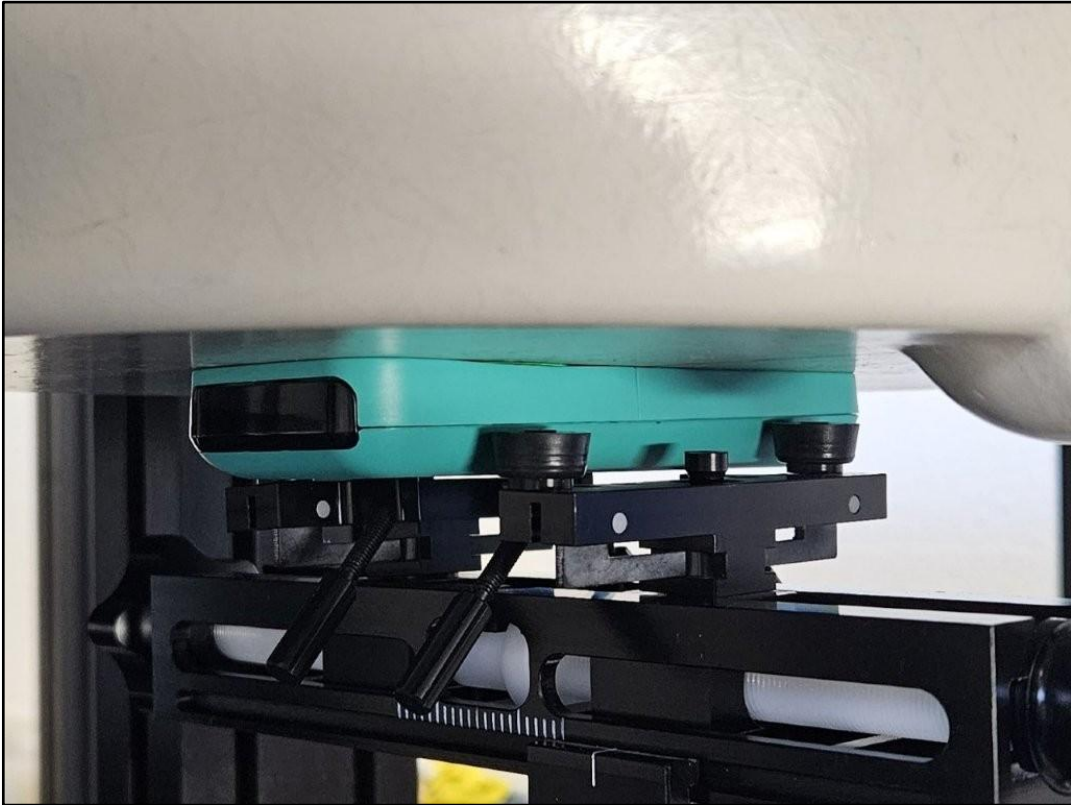
Photo 16: Test position body worn back side with 0 mm distance
