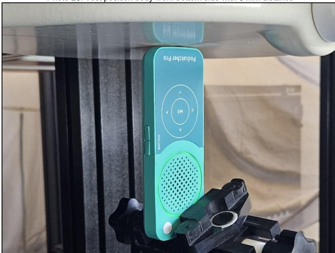
Photo 20: Test position body worn bottom side with 0 mm distance
