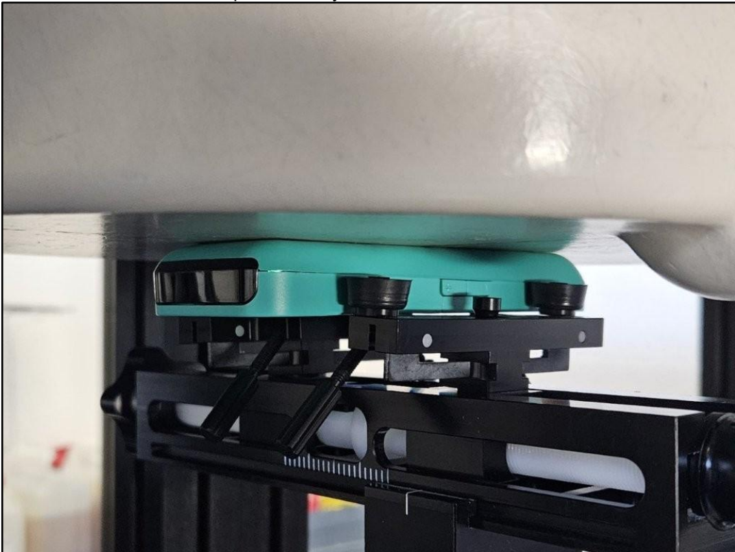
Photo 16: Test position body worn back side with 0 mm distance
