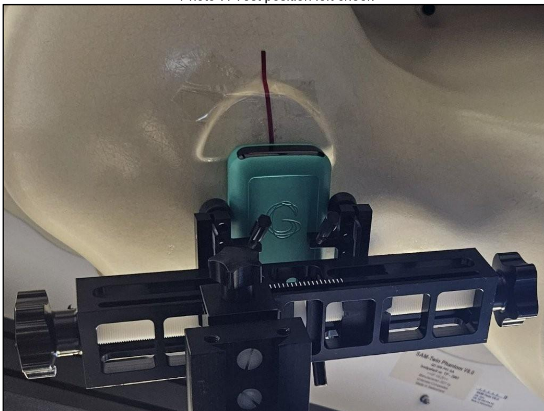
Photo 8: Test position left tilted 15°
