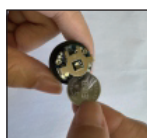
c. Put in a new battery, screw the top cover and install it to the air nozzle (the battery has words facing up)
