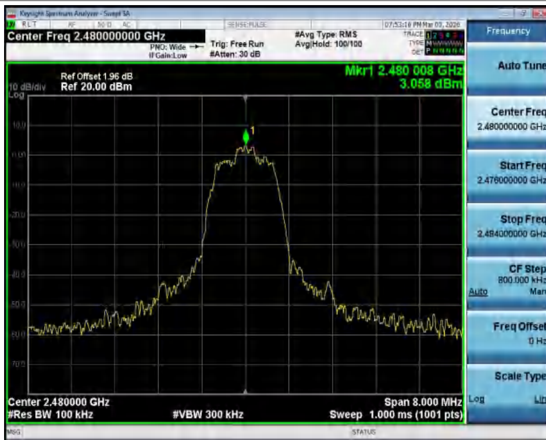
Band Edge NVNT 2-DH1 2480MHz Ant1 No-Hopping Ref
