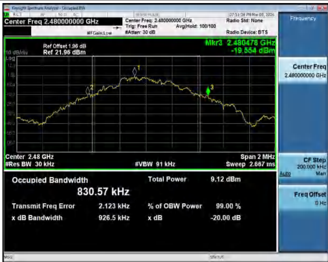
-20dB Bandwidth NVNT 1-DH1 2480MHz Ant1
