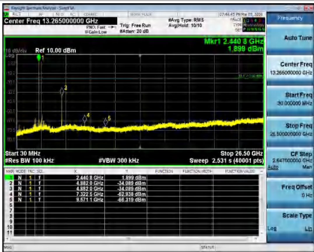
Tx. Spurious NVNT 2-DH1 2441MHz Ant1 Emission
