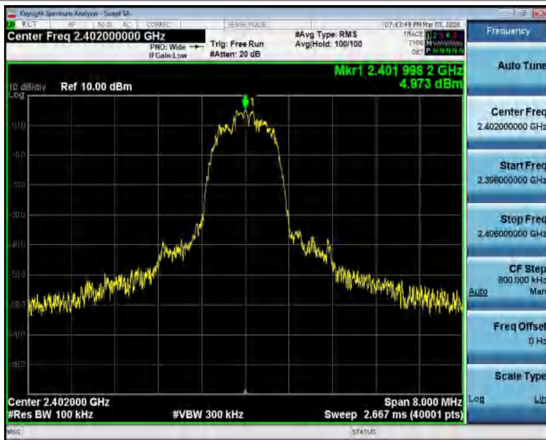
Tx. Spurious NVNT 2-DH1 2402MHz Ant1 Ref
