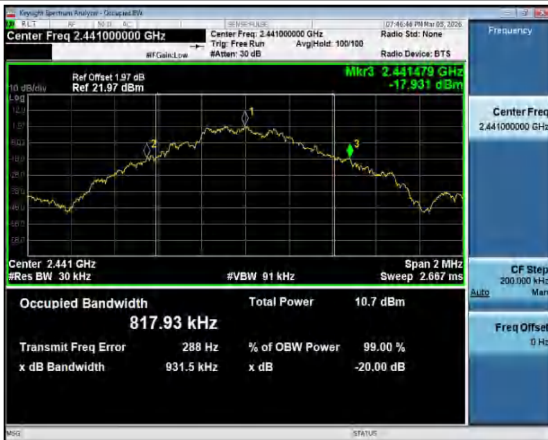
-20dB Bandwidth NVNT 1-DH1 2441MHz Ant1
