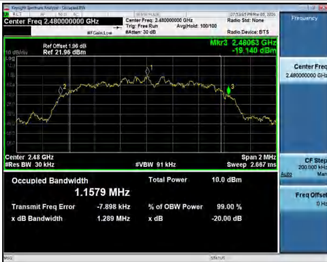
-20dB Bandwidth NVNT 2-DH1 2480MHz Ant1
