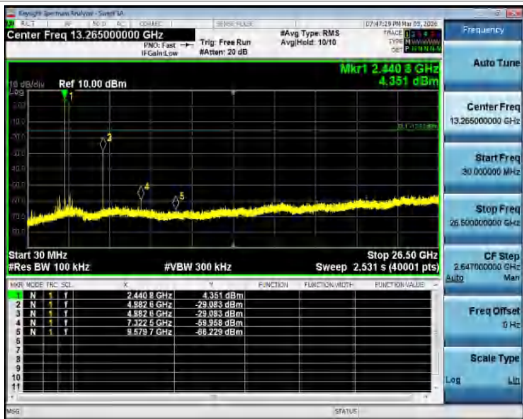
Tx. Spurious NVNT 1-DH1 2441MHz Ant1 Emission
