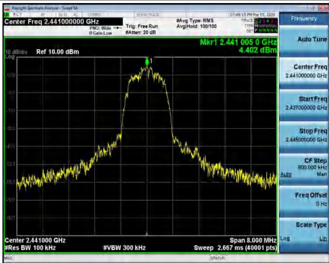
Tx. Spurious NVNT 2-DH1 2441MHz Ant1 Ref
