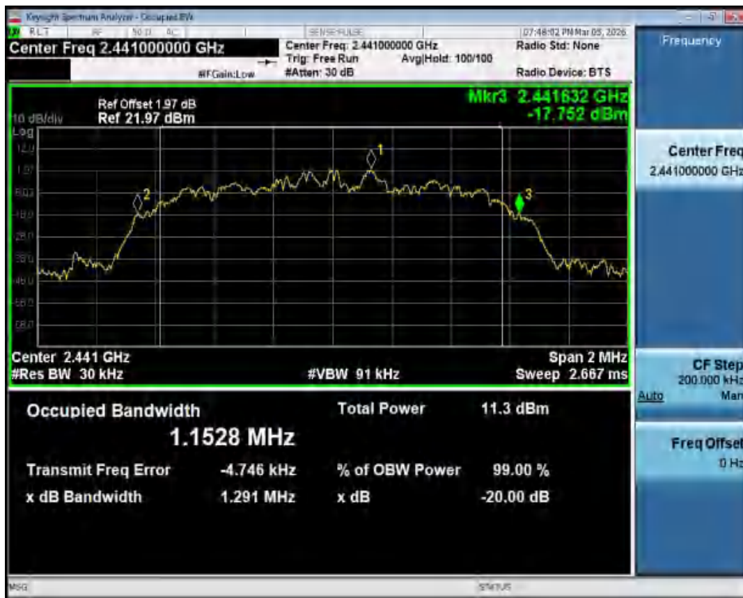
-20dB Bandwidth NVNT 2-DH1 2441MHz Ant1
