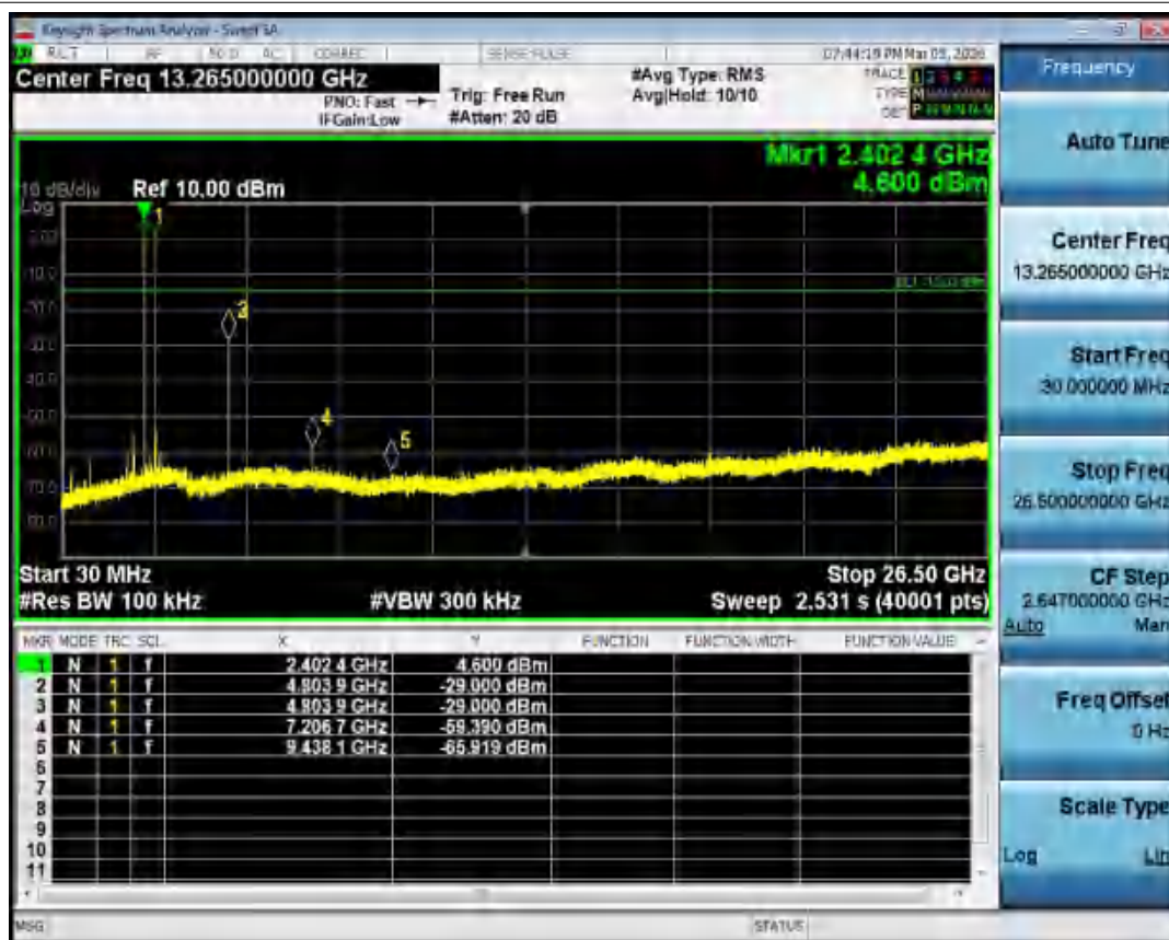
Tx. Spurious NVNT 2-DH1 2402MHz Ant1 Emission
