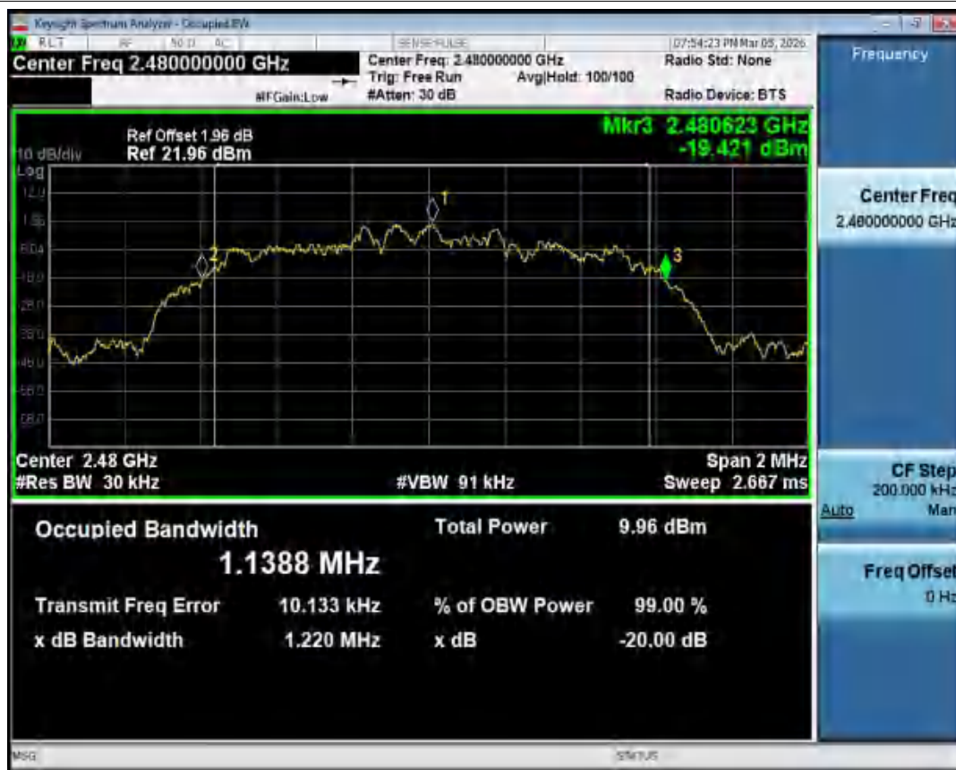
-20dB Bandwidth NVNT 3-DH1 2480MHz Ant1
