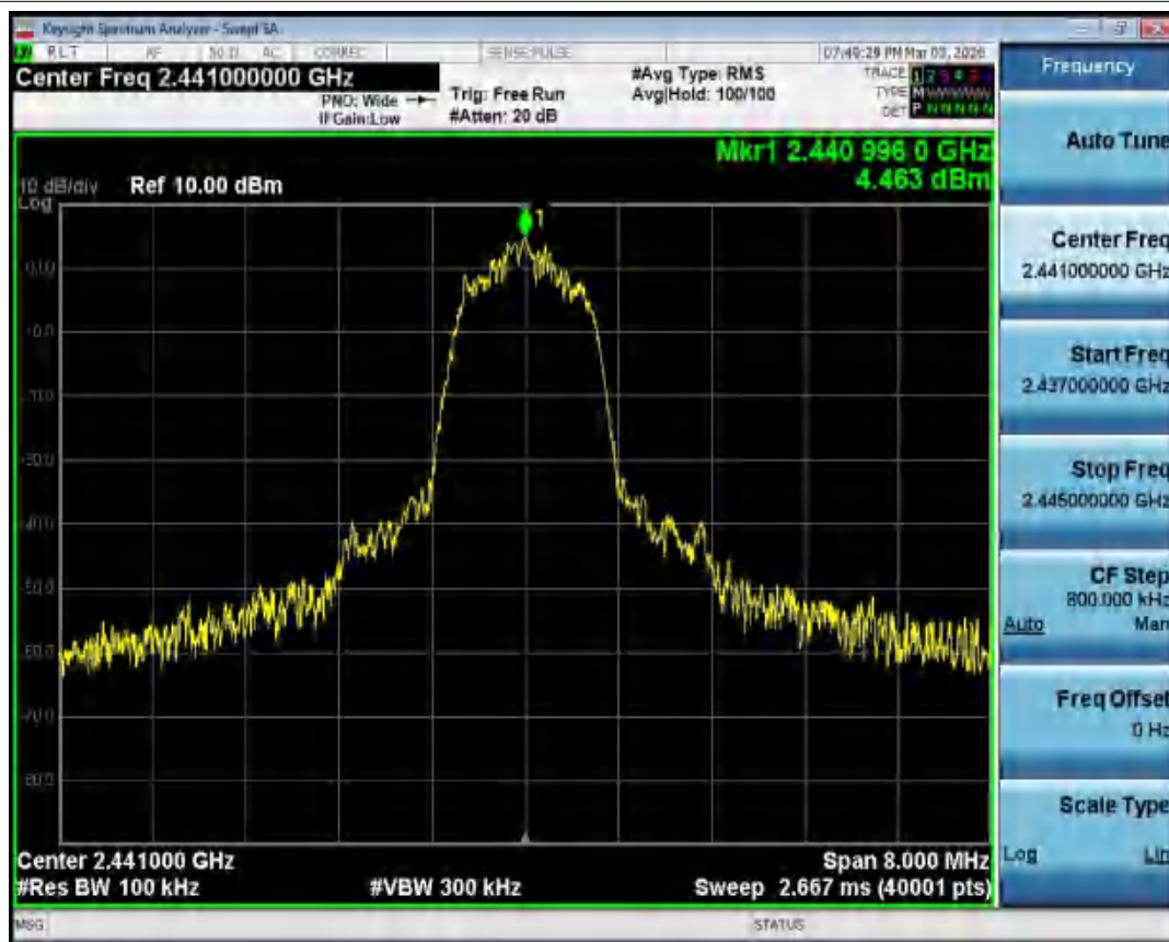
Tx. Spurious NVNT 3-DH1 2441MHz Ant1 Ref
