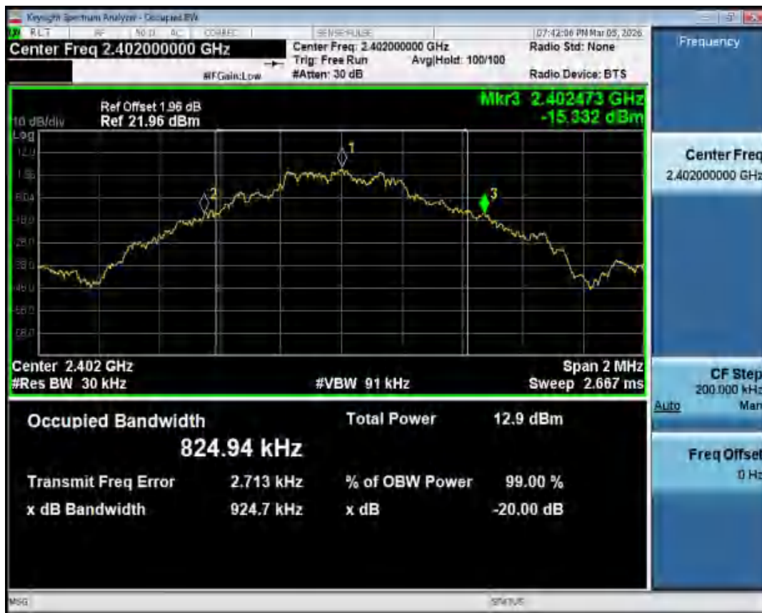
-20dB Bandwidth NVNT 1-DH1 2402MHz Ant1
