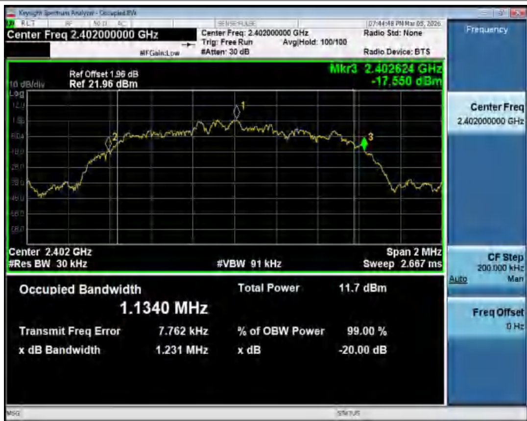
-20dB Bandwidth NVNT 3-DH1 2402MHz Ant1
