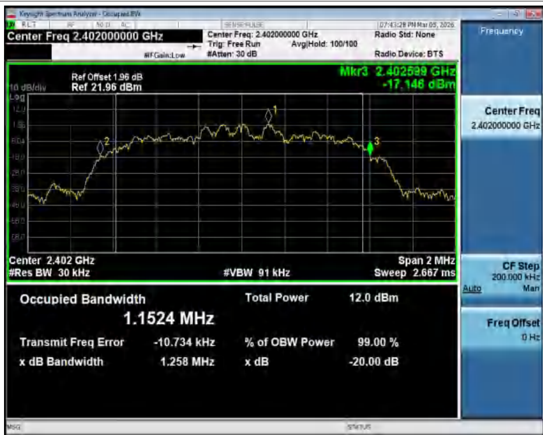
-20dB Bandwidth NVNT 2-DH1 2402MHz Ant1
