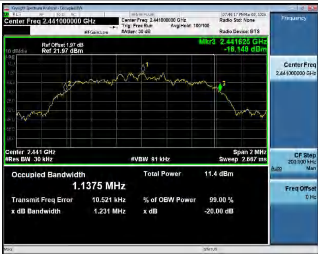
-20dB Bandwidth NVNT 3-DH1 2441MHz Ant1
