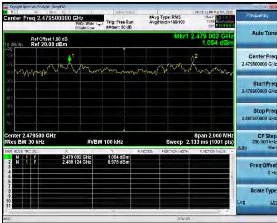
CFS NVNT 2-DH1 2480MHz Ant1
