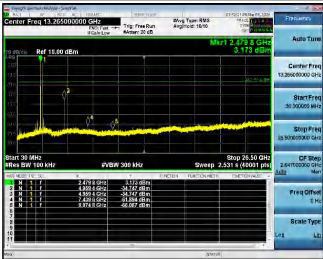
Tx. Spurious NVNT 1-DH1 2480MHz Ant1 Emission
