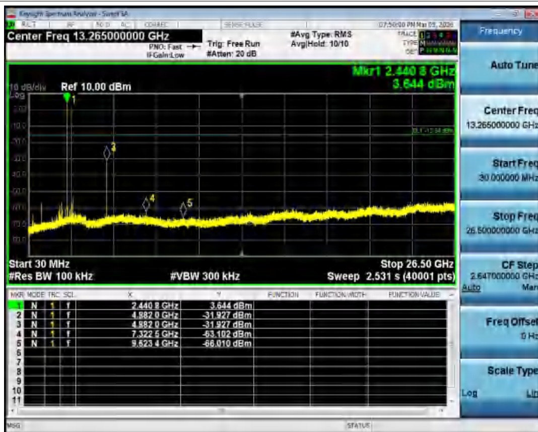
Tx. Spurious NVNT 3-DH1 2441MHz Ant1 Emission
