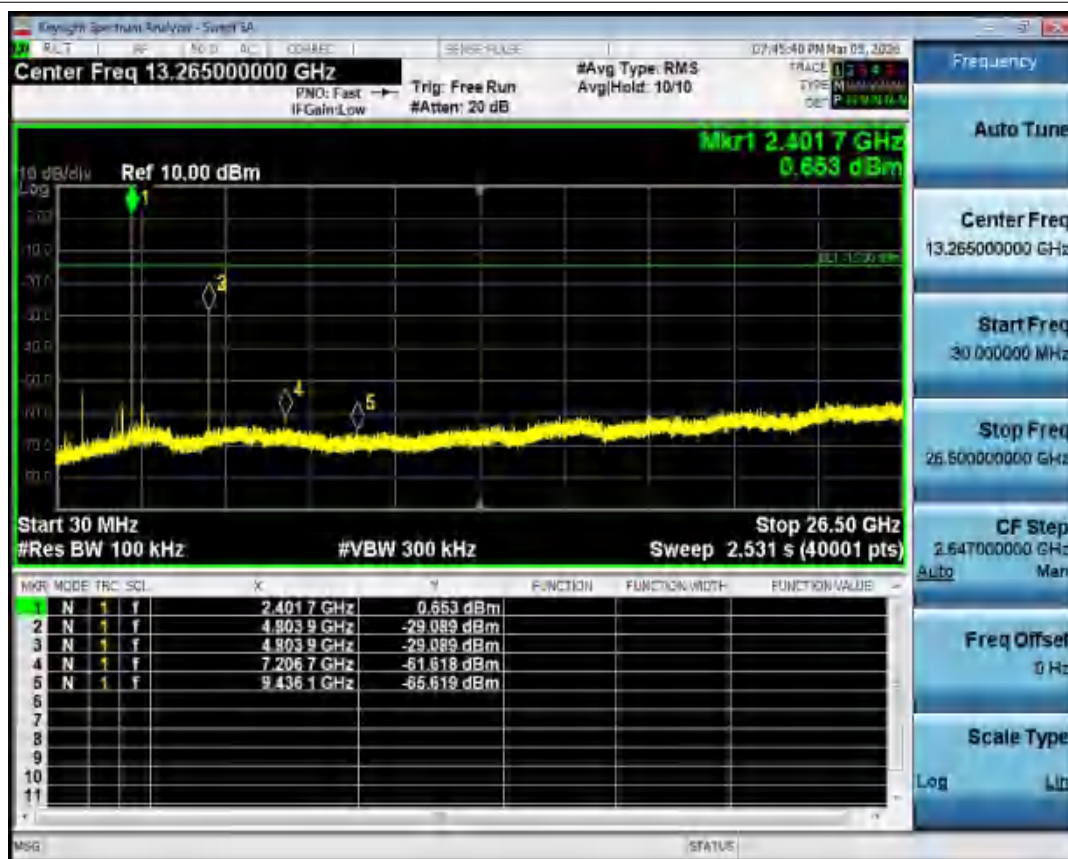
Tx. Spurious NVNT 3-DH1 2402MHz Ant1 Emission
