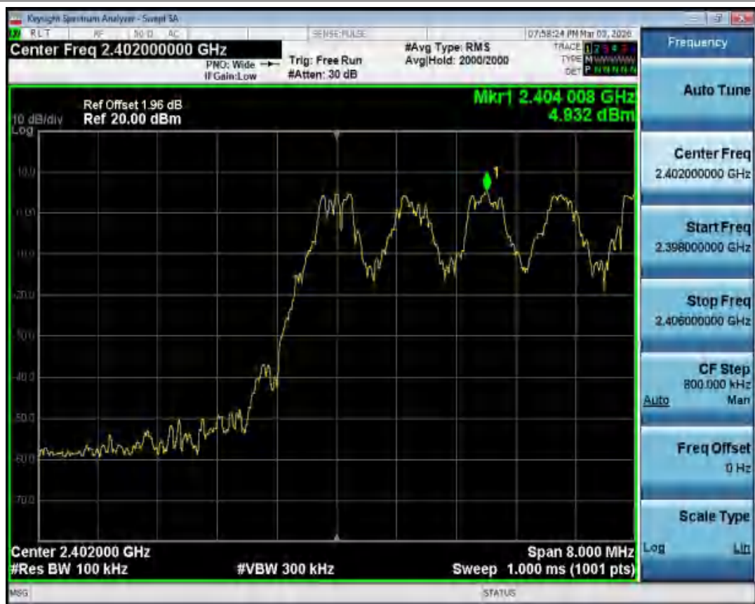
Band Edge(Hopping) NVNT 1-DH1 2402MHz Ant1 Hopping Ref
