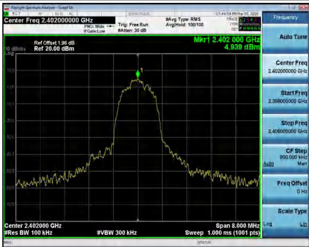
Band Edge NVNT 3-DH1 2402MHz Ant1 No-Hopping Ref
