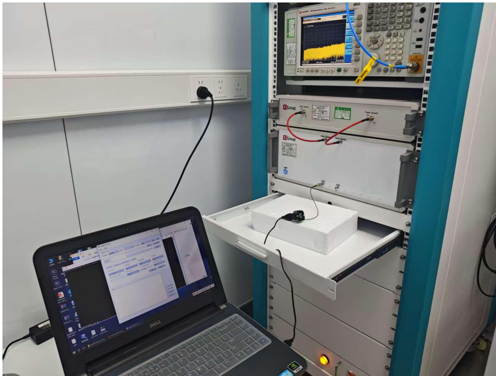
Photo 3 Test Setup Photos of Conducted Test
