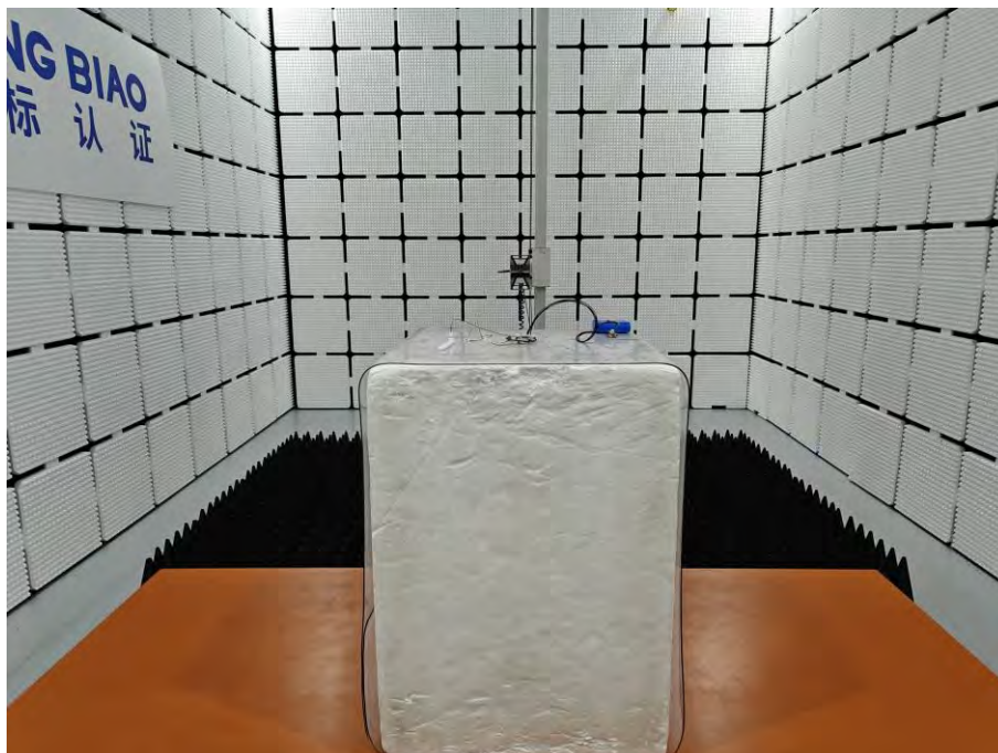
Radiated Emission Above 1GHz
