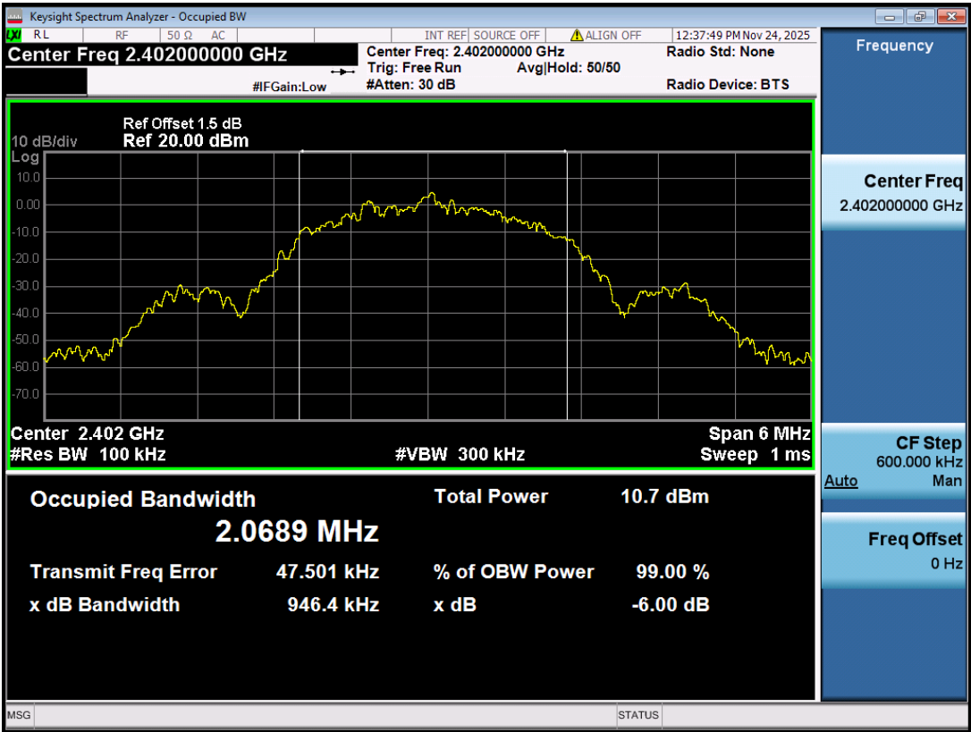
Figure 10: 6dB Bandwidth, 2402MHz, BLE-2Mbps
