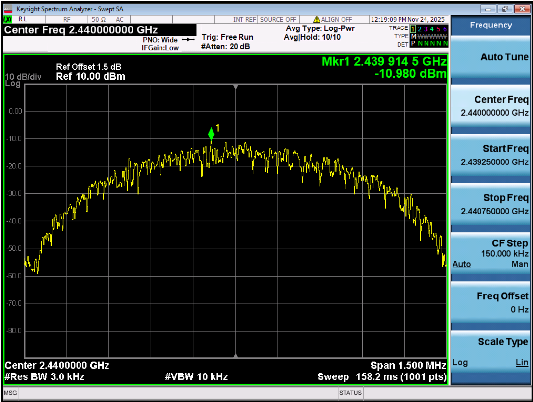
Figure 14: Power Spectral Density, 2440MHz, BLE-1Mbps
