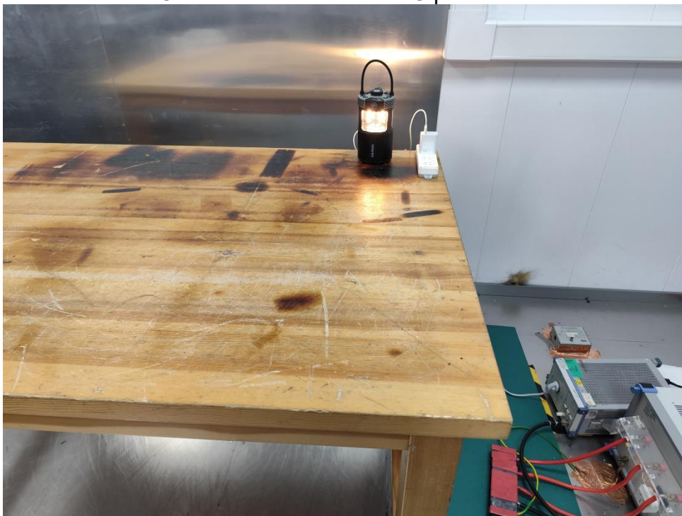
Conducted Emission at AC power line
