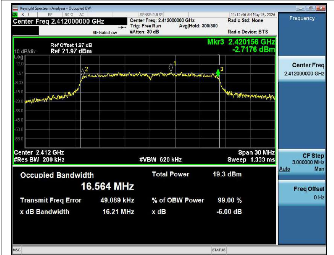
-6dB Bandwidth NVNT g 2412MHz Ant1
