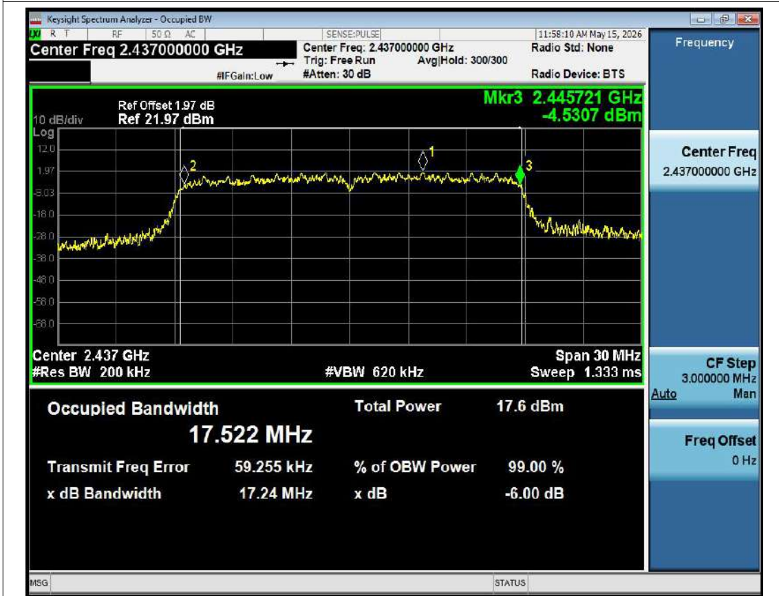
-6dB Bandwidth NVNT n20 2437MHz Ant1
