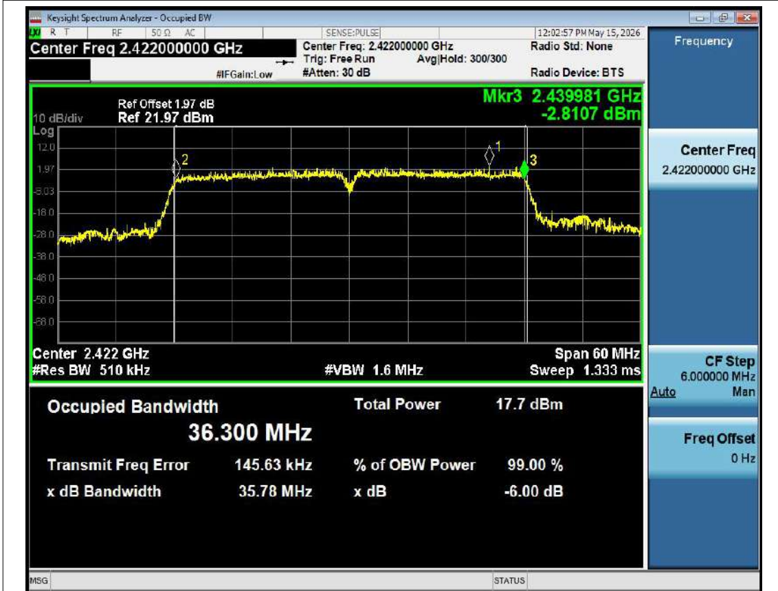
-6dB Bandwidth NVNT n40 2422MHz Ant1
