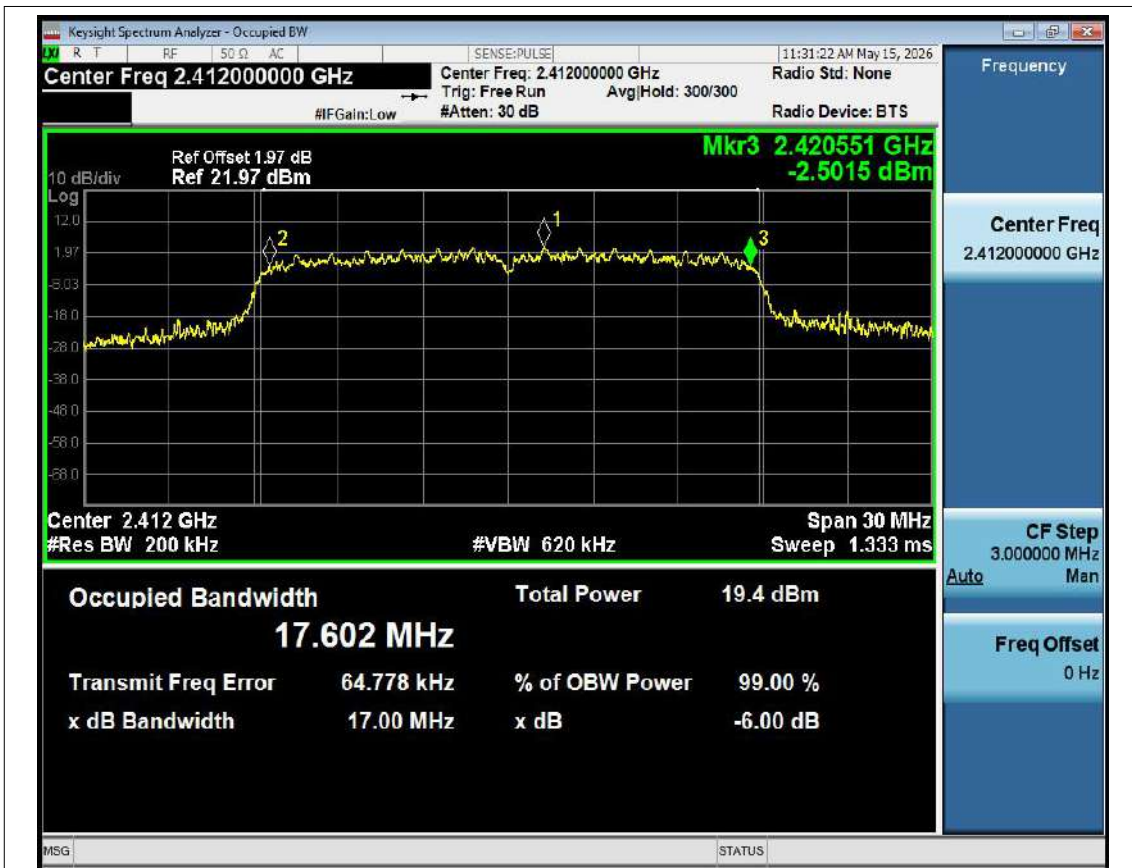
-6dB Bandwidth NVNT n20 2412MHz Ant1
