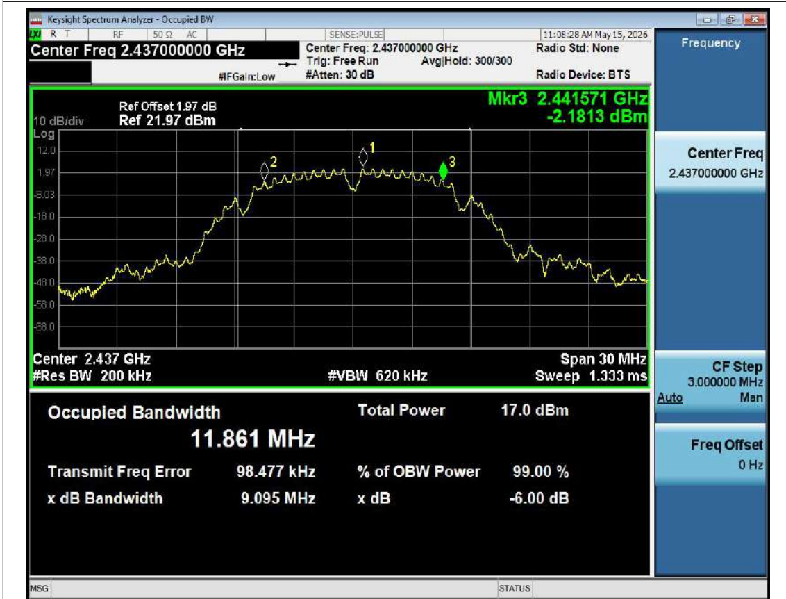
-6dB Bandwidth NVNT b 2437MHz Ant1
