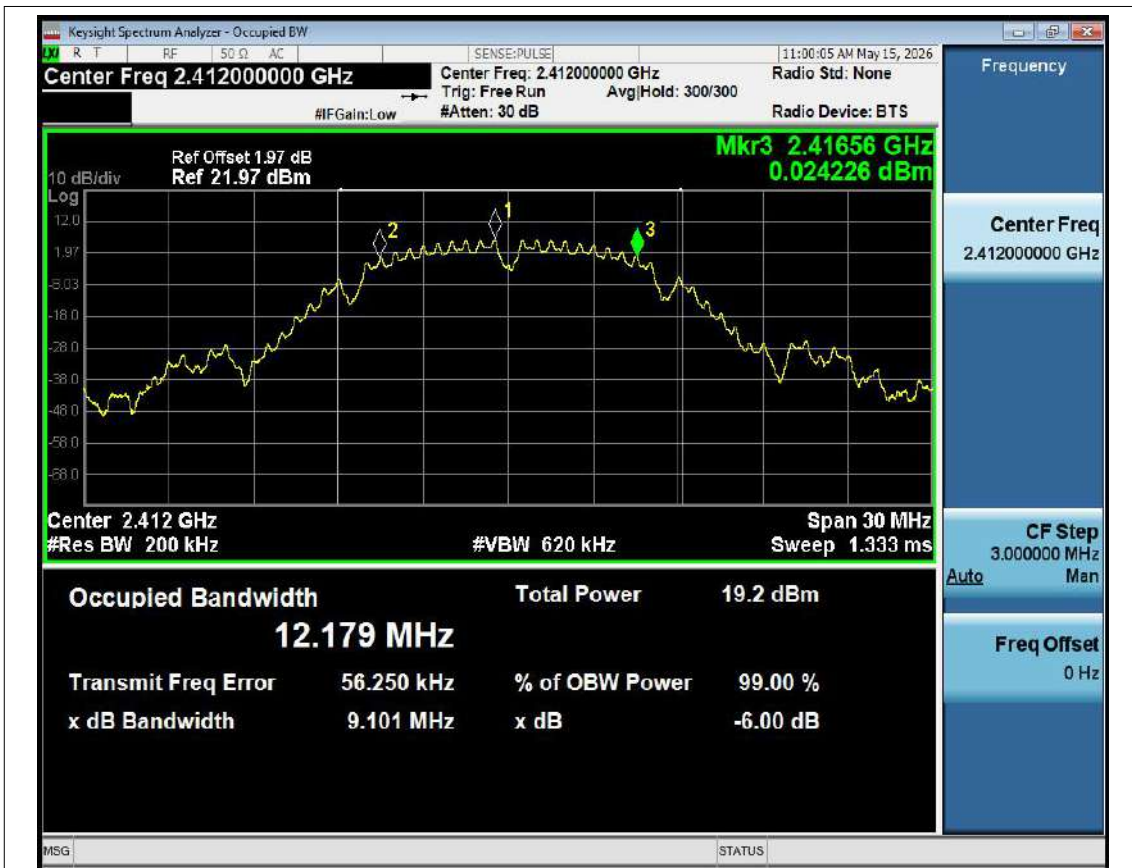
-6dB Bandwidth NVNT b 2412MHz Ant1
